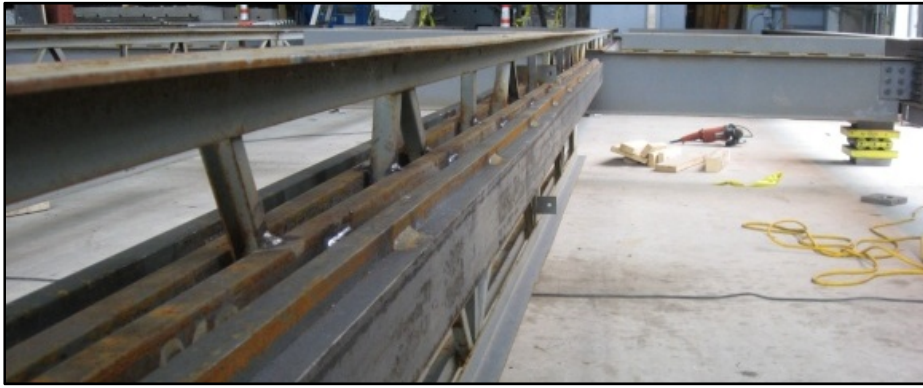
Figure 2.8 – Additional mass in the form of welded steel plates
