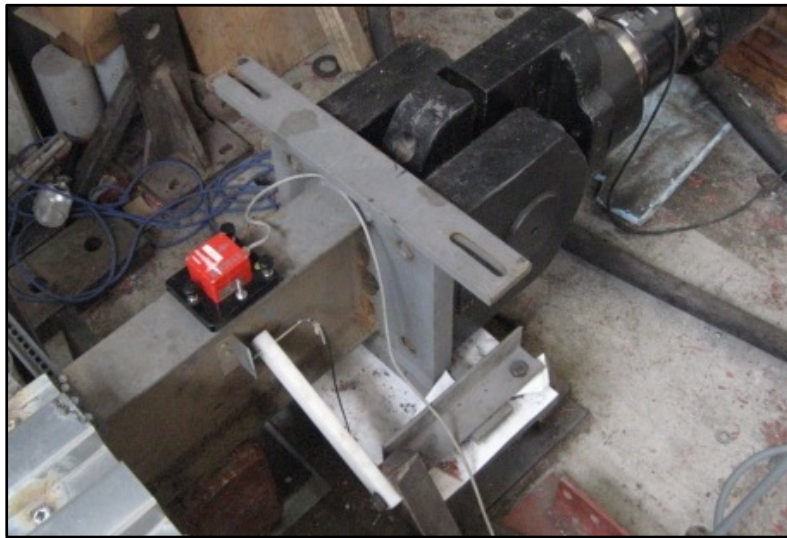
Figure 2.5 – Connection between the actuator's rod end and the end beam extension
