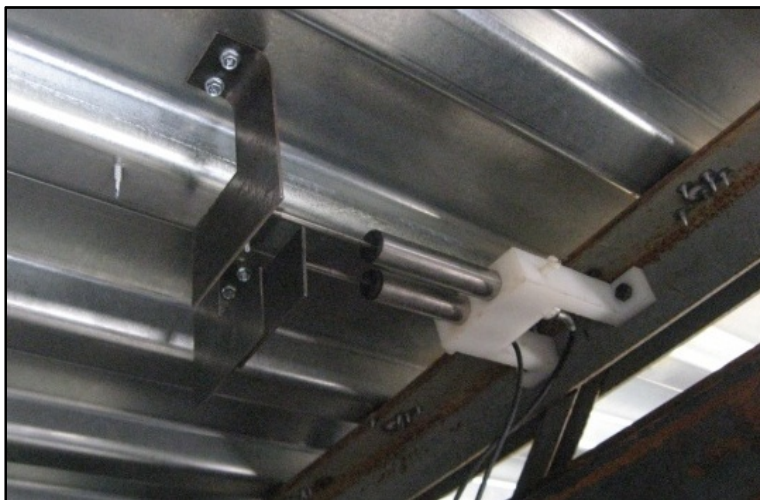
Figure 2.19 – LVDT and Teflon support for sidelap slip measurements
