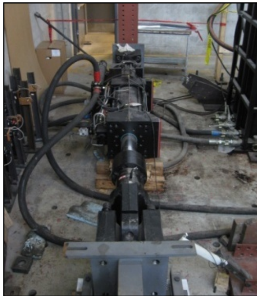
Figure 2.4 – Actuator (black) installed on reaction column (burgundy)
