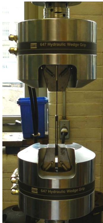
Figure 21: Double-lap sample clamped in the MTS 100kN machine
