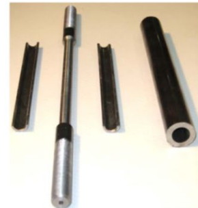
(c) Buckling-restrained axial fuses
