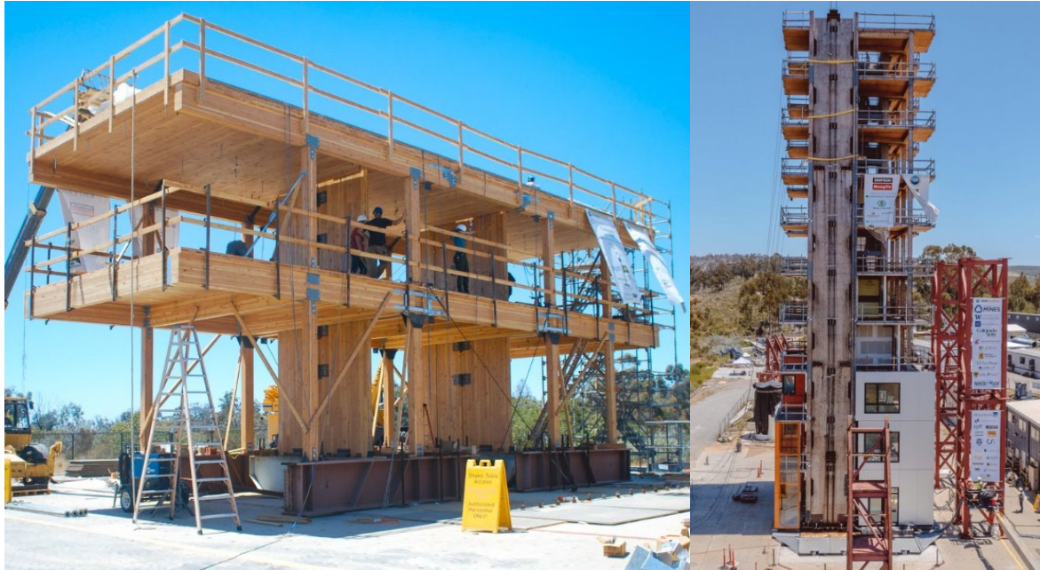
Figure 2-8. Shaking table testing of two-storey (left) and ten-storey (right) PT-CLT shear wall buildings. (Picture source: https://leverarchitecture.com/innovation ).
