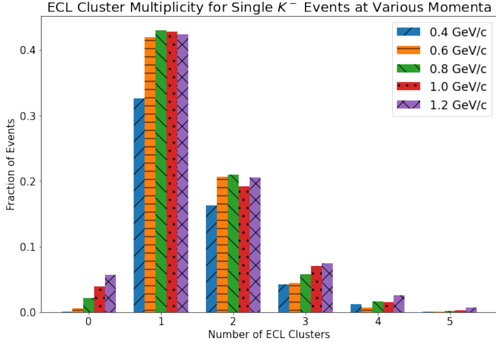
Figure 5.8: ECL multiplicity for simulated single negative kaon events at various momenta. The momentum for each distribution can be found in the legend.
