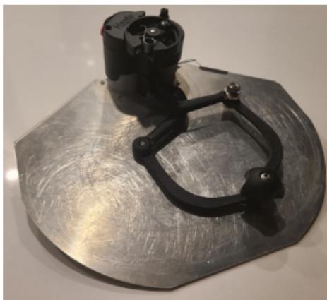
(a) The Haply 2diy device used for force-feedback, showing the end-effector extended towards the bottom of the plate.
