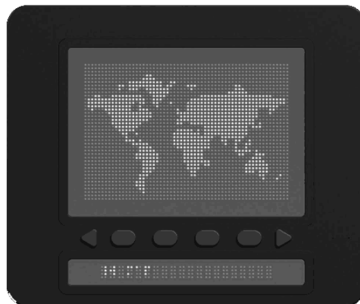
(b) The Dot Pad device (image taken from https://web.archive.org/web/20230410040328/https://pad.dotincorp.com/ ).
