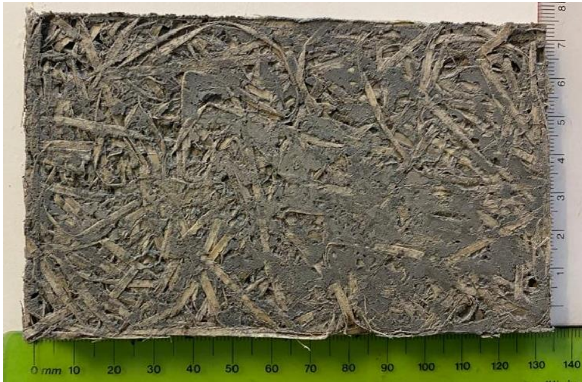
Figure 0-3 Photo of slag bonded strand board (12.7 * 7.6 * 1.3 cm).
