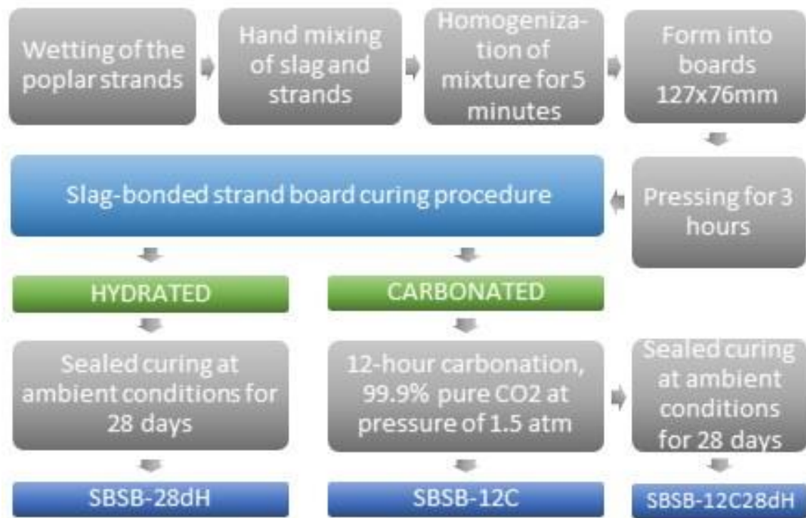
Figure 4-2 Manufacturing process of slag-bonded strand board (SBSB).
