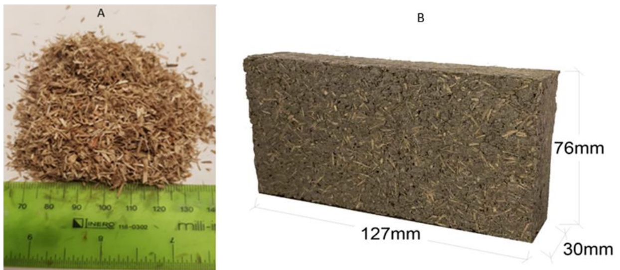
Figure 5-2 (A) Recycled wood aggregates, (B) Typical wood-SMU.
