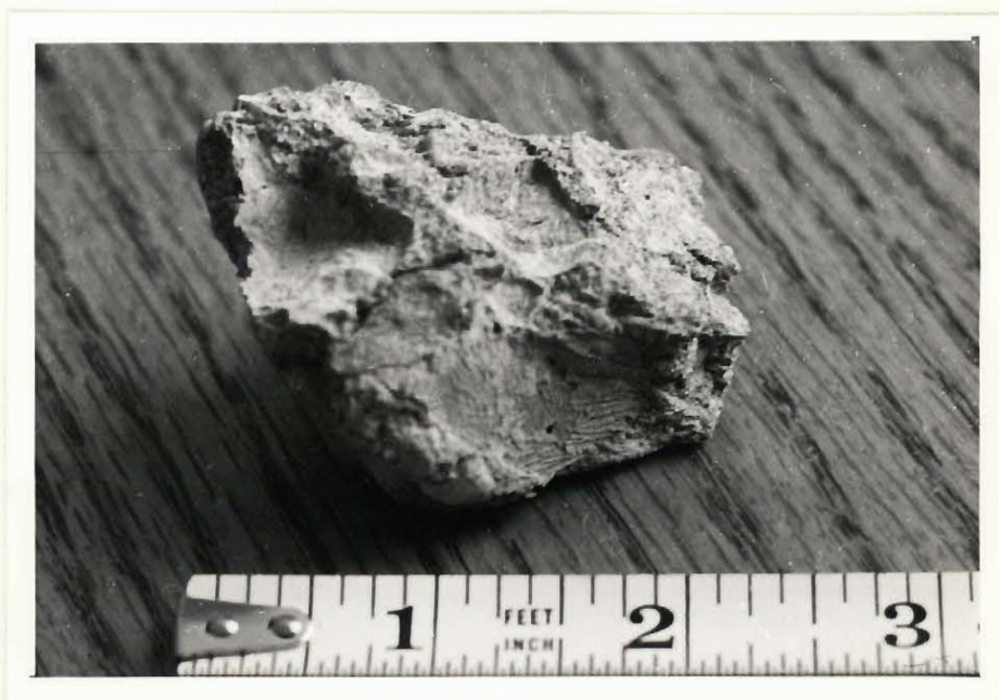
Figure 7. Rupture of the mortar in frozen concrete.
