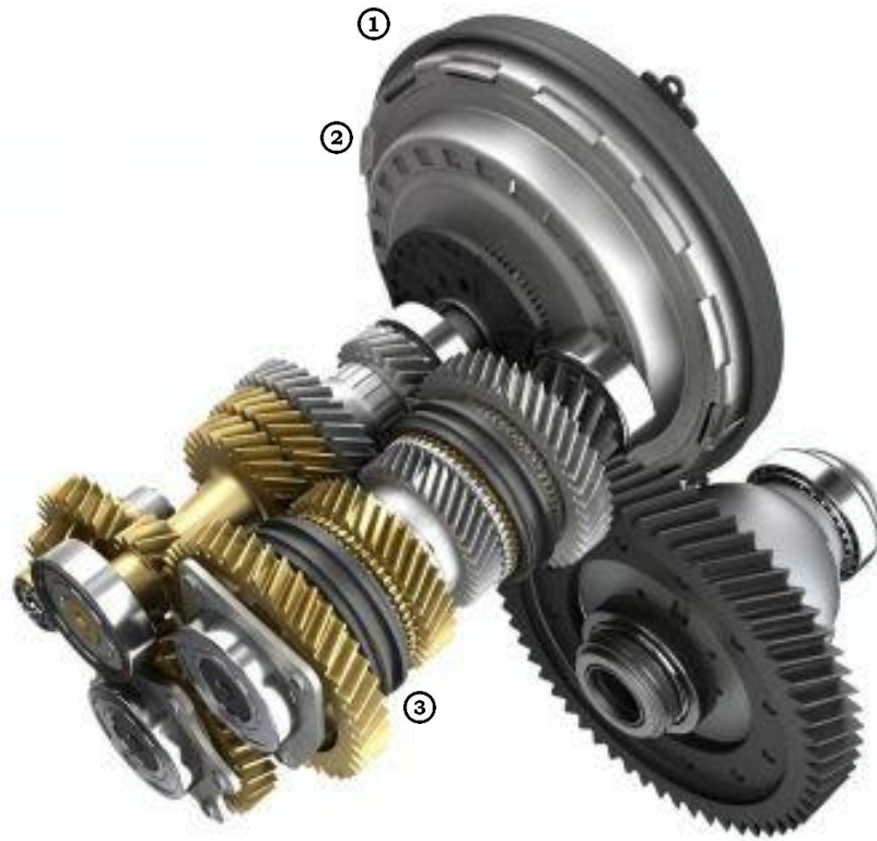
Figure 1.2 Manual transmission components: flywheel (1), clutch (2), and gears (3) [12]
