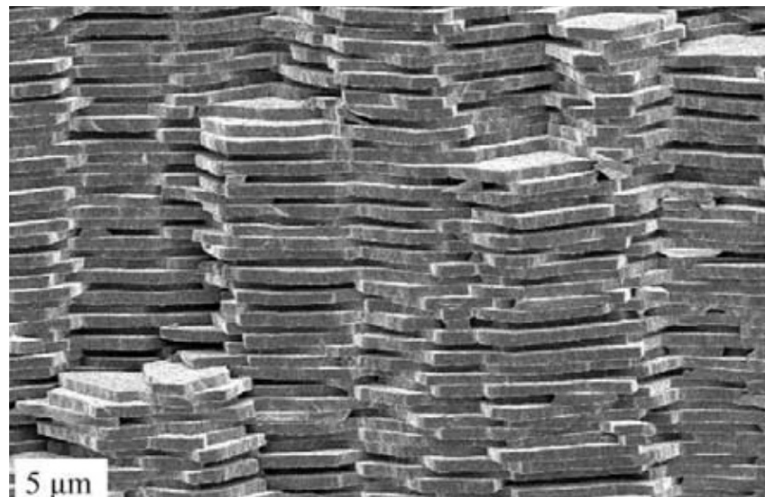
Figure 2.1: Microscopic view of microtablets arrangements in nacre [71].
