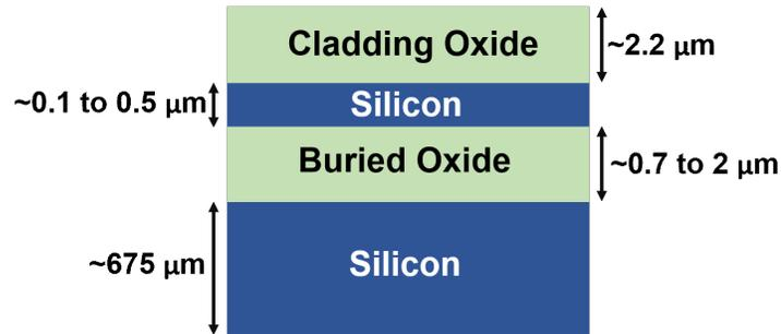
Fig. 2.1 Schematic of the cross-section of a silicon-on-insulator wafer [5].
