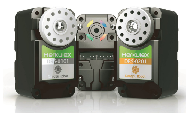
Fig. 2.20 Dongbu HerkuleX DRS-0101 and DRS-0201 (HerkuleX manual)
