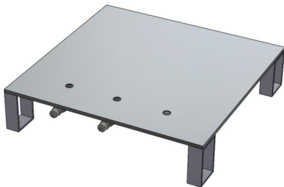
Figure 3.1-1: HTP trimetric view showing tool surface, vacuum fittings, and support structure
