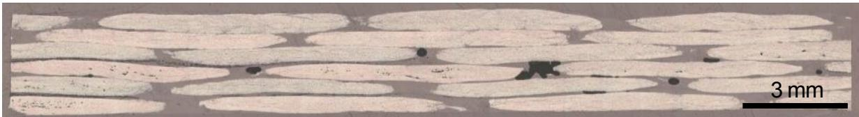
Figure 6.1-4: RFI trial 5 sample micrograph, 2.31 % void content
