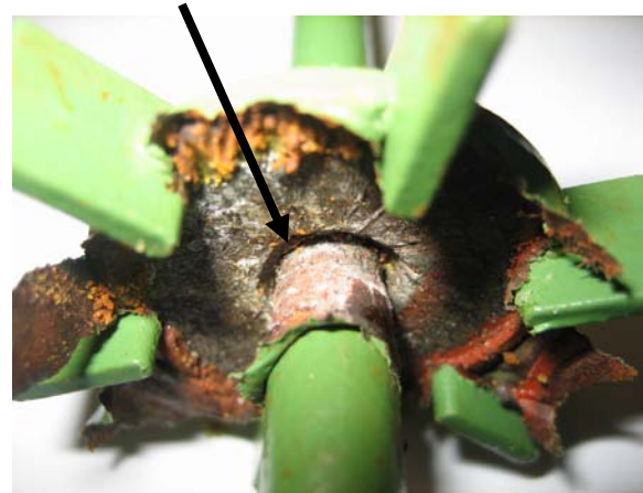
Figure 29: Crevice corrosion at the stirrer (Teflon coating removed).
