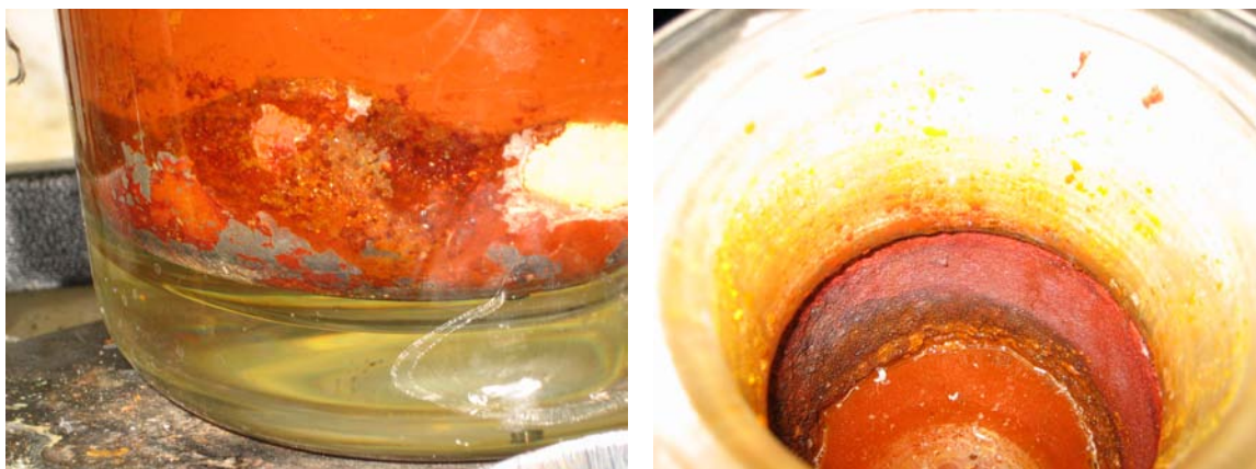
Figure III.5: Scale formation inside the reactor (RT38).
