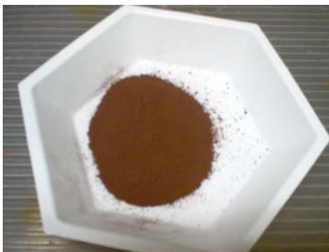
Figure I.3: Thermal Composition Product (FeOCl) after Grinding.
