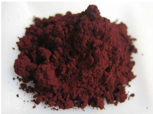
Figure 22: Image of the Precipitated Hematite by Oxidation at 150°C (RT56).
