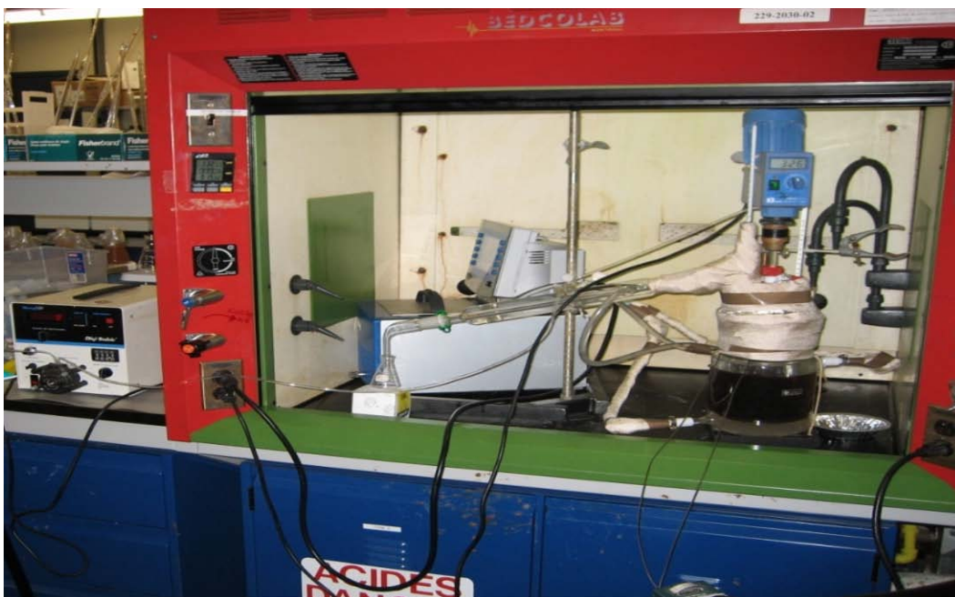
Figure 18: Experimental Setup of Hydrolytic Distillation.
