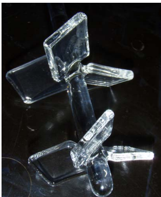
Figure 17: Glass Stirrer with Dual Impellers and Dimensions (in cm).
