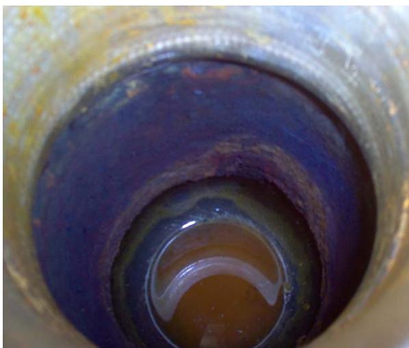
Figure 36: Scale in the Reactor after the Removal of the Reaction Products (RT42).
