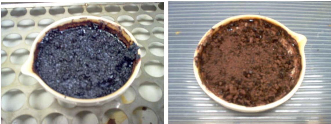
Figure I.2: Picture of the Solid Phase (FeOCl) obtained after 44 h Heat Treatment at 100 °C (Note: The picture on the Right was taken after Agitating the solid with a Spatula).
