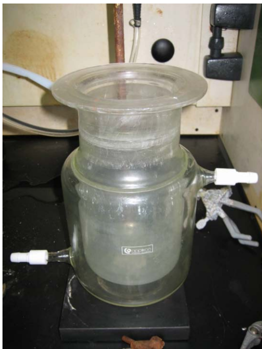
Figure 13: Double Wall Applicon® Glass Reactor (1.6L volume capacity) with Dimensions (in cm).
