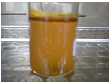
Figure I.6: Hydrothermal Transformation of FeOCl to \beta -FeOOH after 2 Hours Heating at 100°C.
