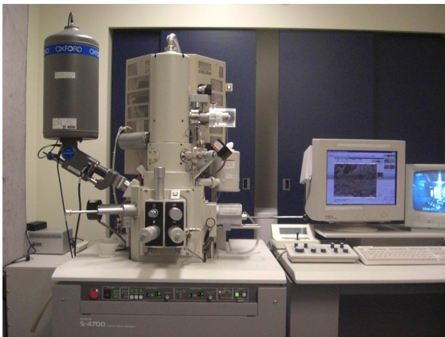
**Figure 3.10** Hitachi S-4700 field-emission gun Scanning Electron Microscopy.
