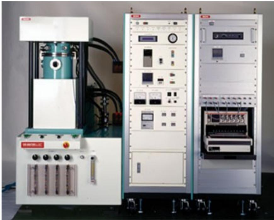
**Figure 3.4** Spark Plasma Sintering (SPS) system.
