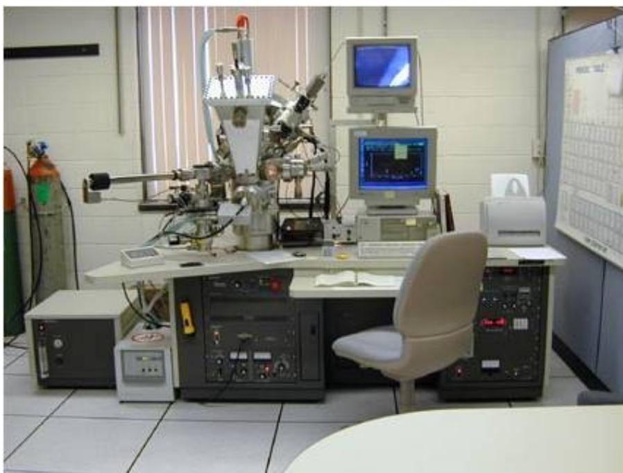
**Figure 3.12** PHI-5700 X-ray Photoelectron Spectrometer
