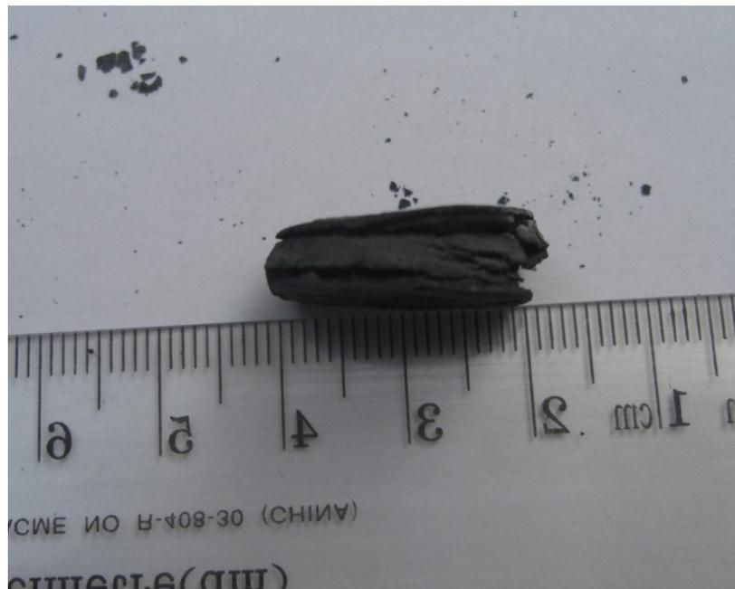
**Figure 8.6** Hot pressed 316LSS samples oxidized at 1000 °C showing complete spallation of its structure.
