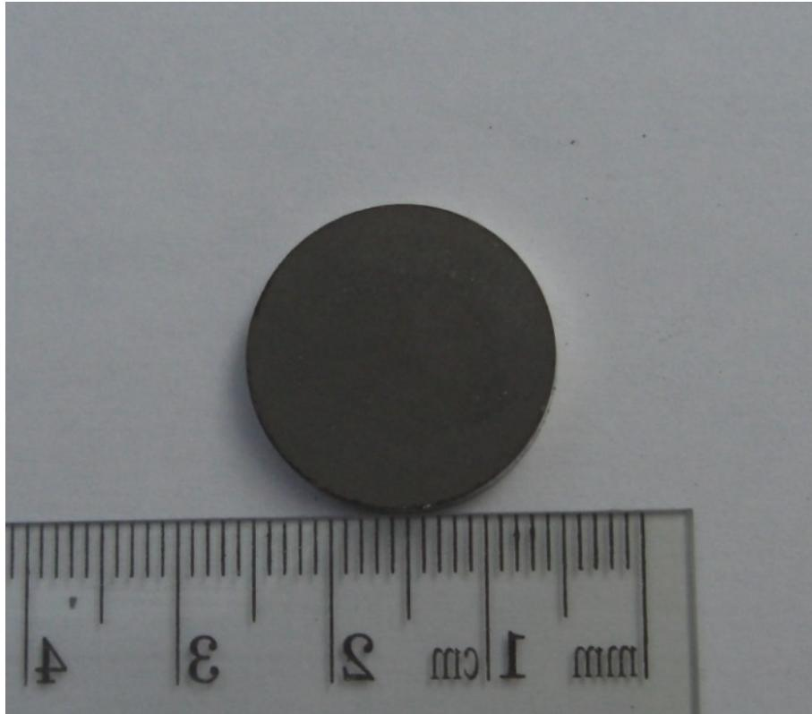
**Figure 3.3** The consolidated powders prior the oxidation test
