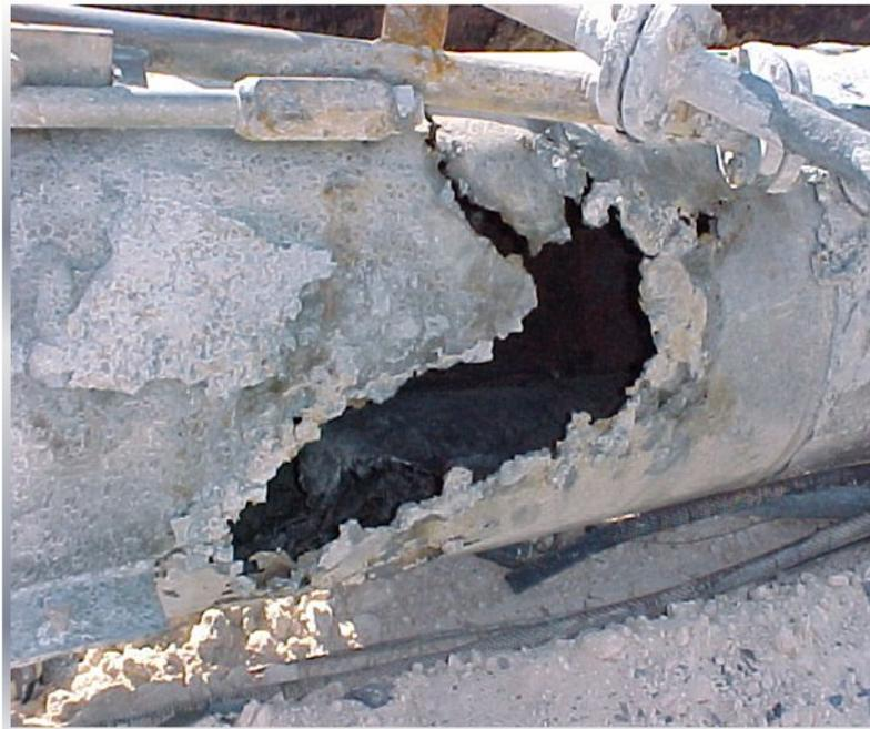
**Figure 1.1** Tube failure in one of Aramco oil and gas operations due to high temperature corrosion.
