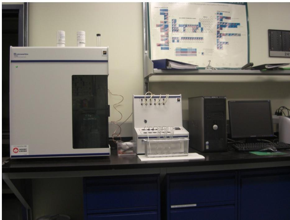
**Figure 3.5** Micromeritics Tristar 300 BET instrument.
