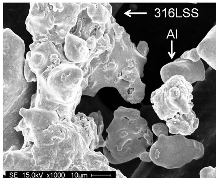
**Figure 5.1** SEM image of stainless steel 316L and Al mixed powders, before cryomilling.
