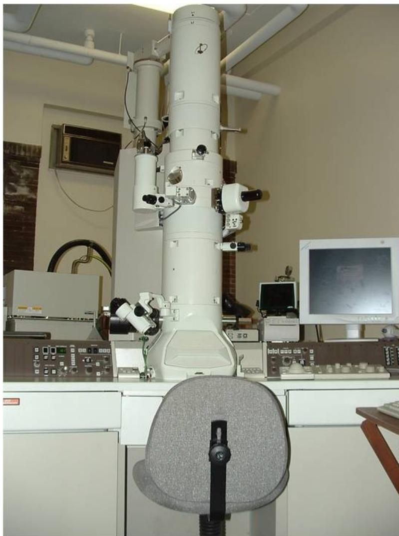
**Figure 3.11** JEOL JEM-2011 Transmission Electron Microscopy
