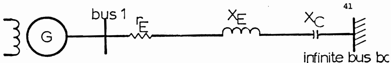
(a) Synchronous generator connected to an infinite bus through a series capacitor compensated transmission line.
