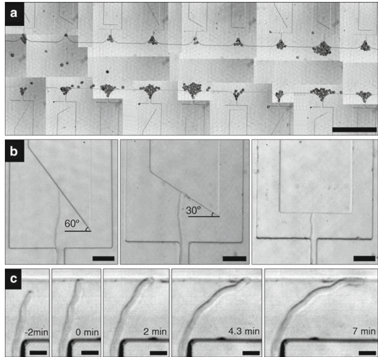
Fig. 3 Mechanical obstacle test. (a) Initial pollen grain distribution (image is stitched from several high-magnification micrographs. Scale bar = 1 mm. (b) Pollen tubes colliding with flat wall oriented at 60°, 30°, and 0° relative to the growth direction. Scale bars = 100 \mu\text{m} . (c) Time-lapse sequence of a type 0° collision. Scale bars = 25 \mu\text{m} . Reproduced from [11] with permission from IOP Publishing Limited
