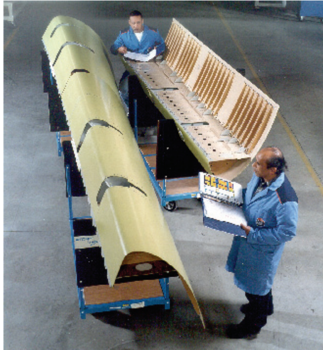
Fig. 1-2. J-nose leading edge of Airbus A340/600 airplane, courtesy of Stork Fokker
