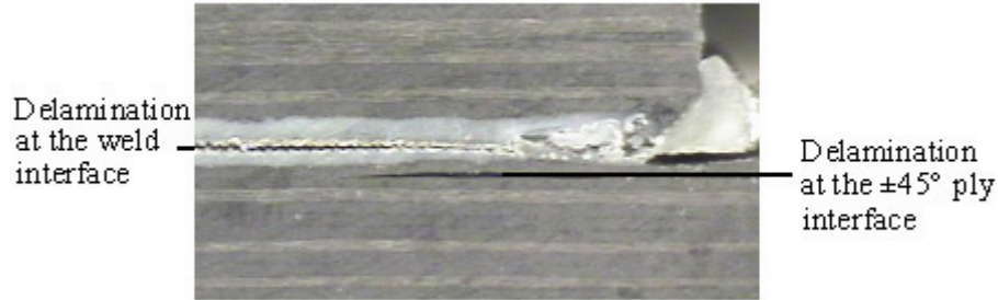
Fig. 5-12. Failure mode of the quasi-isotropic specimens welded using the \text{TiO}_2 HE
