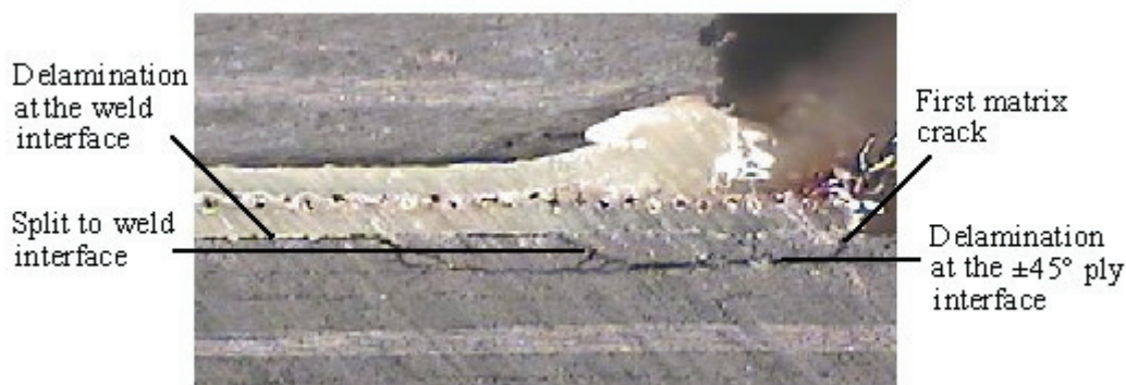
Fig. 5-9. Failure mode of the quasi-isotropic specimens welded using the uncoated HE
