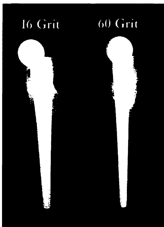
Figure 5-7 Matched 16 and 60 grit specimens. New bone formation is clearly visible at the distal end of the implant.
