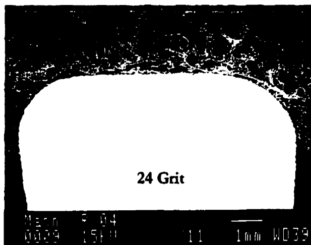
Figure 5-31 24 Grit stem. Dense interconnected trabecular bone and large extent of apposition.
