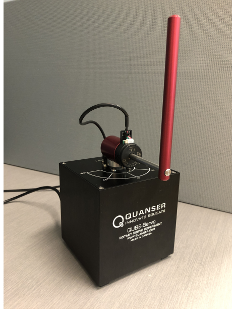
Figure 6.6: The Quanser QUBE-Servo system used to demonstrate the proposed closed-loop Koopman operator approximation method.
