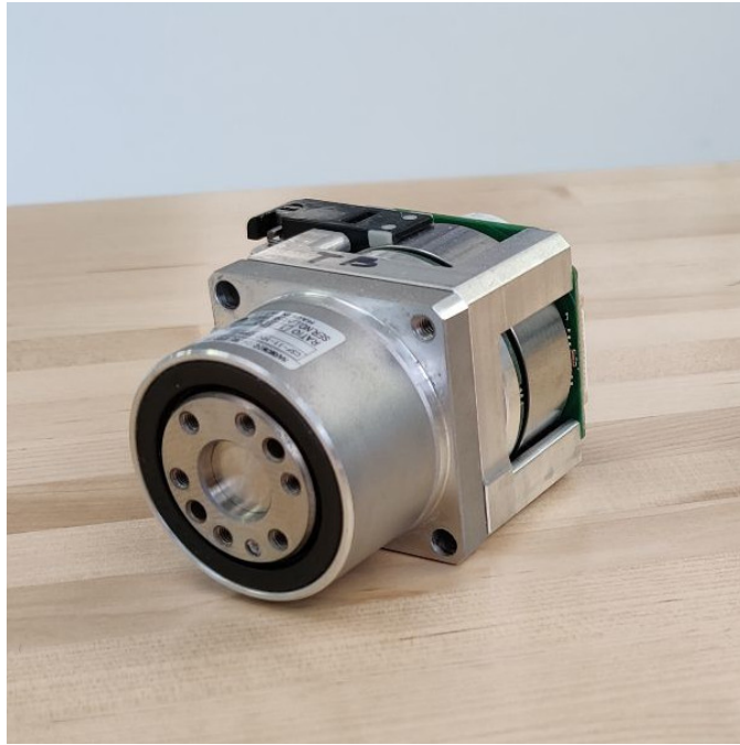
Figure 7.8: Motor drive used to generate the training data, which consists of a motor with a Harmonic Drive gearbox. The gearbox introduces nonlinear oscillations into the system, leading to tracking errors at specific frequencies related to the input velocity. Photo courtesy of Alexandre Coulombe.
