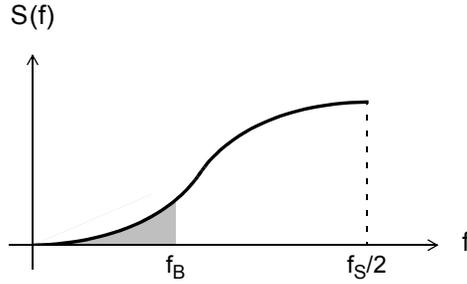
**Figure 2.7:** Power spectral density of the quantization error in a noise-shaping ADC.
