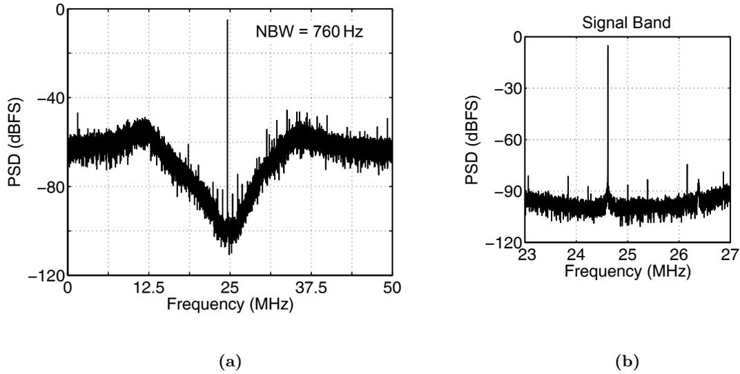
**Figure 8.6:** Measured output spectrum of the experimental  $\Delta\Sigma$  modulator for a  $-5$  dBFS input tone at 224.6 MHz: (a) from 0 to  $f_S/2$ , and (b) over the signal band.
