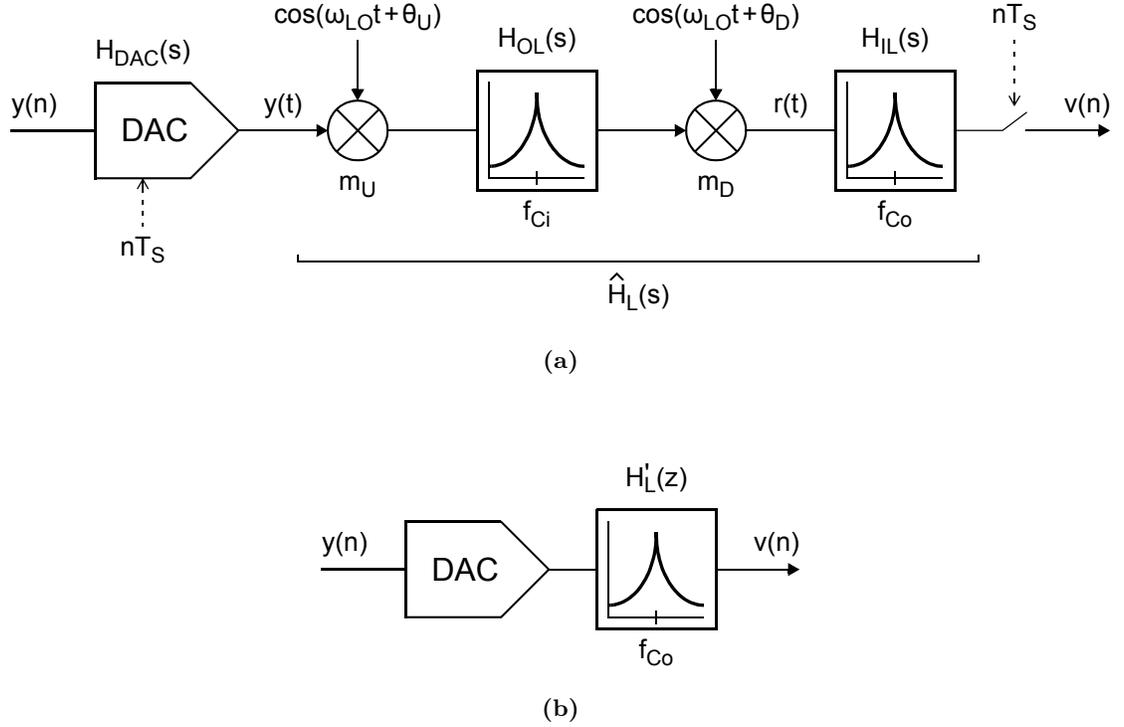
**Figure 5.4:** The loop feedback paths of: (a) the single-path frequency-translating  $\Delta\Sigma$  modulator in Figure 5.1, and (b) the equivalent discrete-time bandpass  $\Delta\Sigma$  modulator in Figure 5.3.
