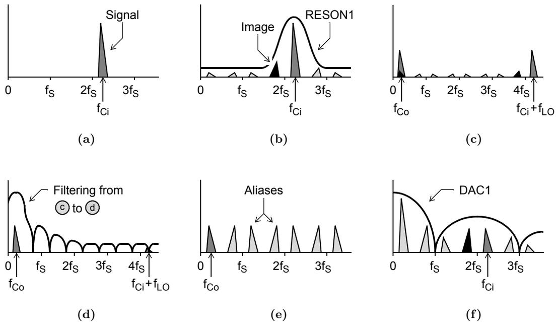
**Figure 6.2:** Frequency spectrum at various points around the feedback loop of the experimental  $\Delta\Sigma$  modulator, shown in Figure 6.1.
