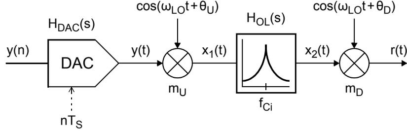
**Figure 5.9:** The outer-loop path of a single-path frequency-translating  $\Delta\Sigma$  modulator.
