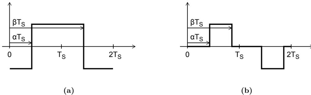
**Figure 3.6:** Timing diagrams for: (a) an NRZ pulse, and (b) an RZ pulse.
