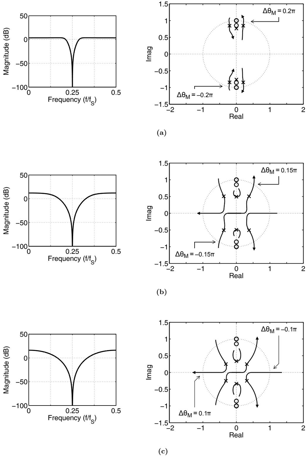
**Figure 5.16:** Root locus plots that illustrate the shift in the NTF poles of a frequency-translating  $\Delta\Sigma$  modulator when the relative LO phase ( $\theta_M$ ) is varied from its nominal value. Here, the out-of-band gain is set to: (a) 3.5 dB, (b) 12.0 dB, and (c) 16.3 dB.
