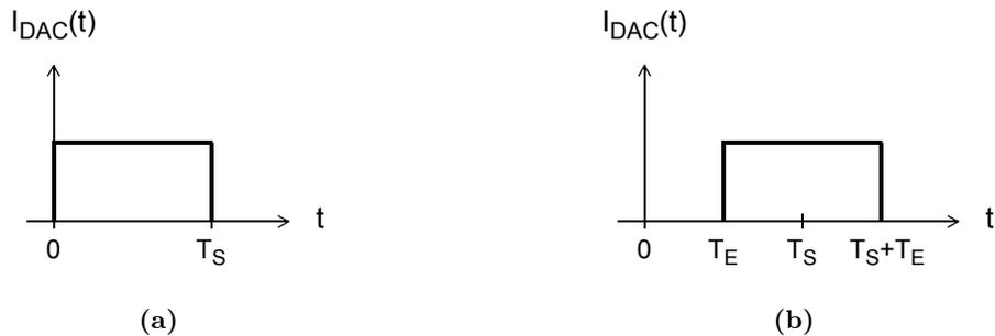
**Figure 3.2:** (a) An ideal non-return-to-zero (NRZ) DAC pulse, and (b) the DAC pulse shown in (a) with an excess loop delay of  $T_E$ .
