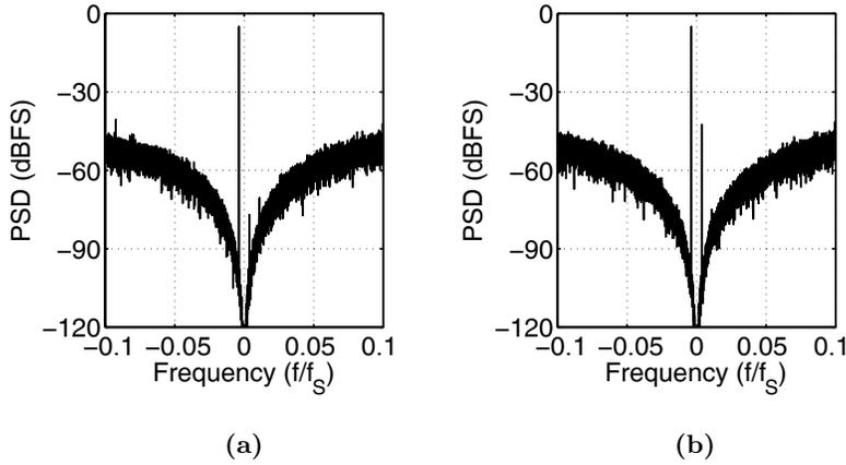
**Figure 4.12:** The output spectrum of the test architecture shown in Figure 4.8, when it is designed with  $T_S = 3T_{LO}/2$  and  $T_D = T_S/2$ . Here, a phase error of  $\Delta\theta$  is introduced into the LO signal that is applied to the quadrature mixer in the *forward* path, where: (a)  $\Delta\theta = 0.0015\pi$ , and (b)  $\Delta\theta = 0.15\pi$ .
