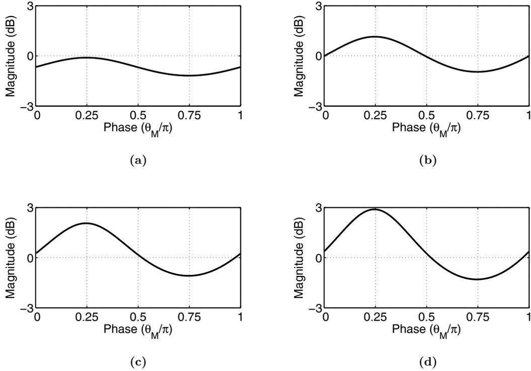
**Figure 5.17:** The STF gain, as a function of  $\theta_M$ , at the input centre frequency ( $f_{Ci}$ ) of a single-path frequency-translating  $\Delta\Sigma$  modulator for: (a)  $k_S = 1$ , (b)  $k_S = 2$ , (c)  $k_S = 3$ , and (d)  $k_S = 4$ .
