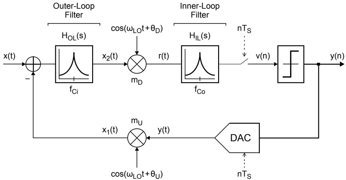
**Figure 5.1:** Block diagram for a single-path frequency-translating  $\Delta\Sigma$  modulator.
