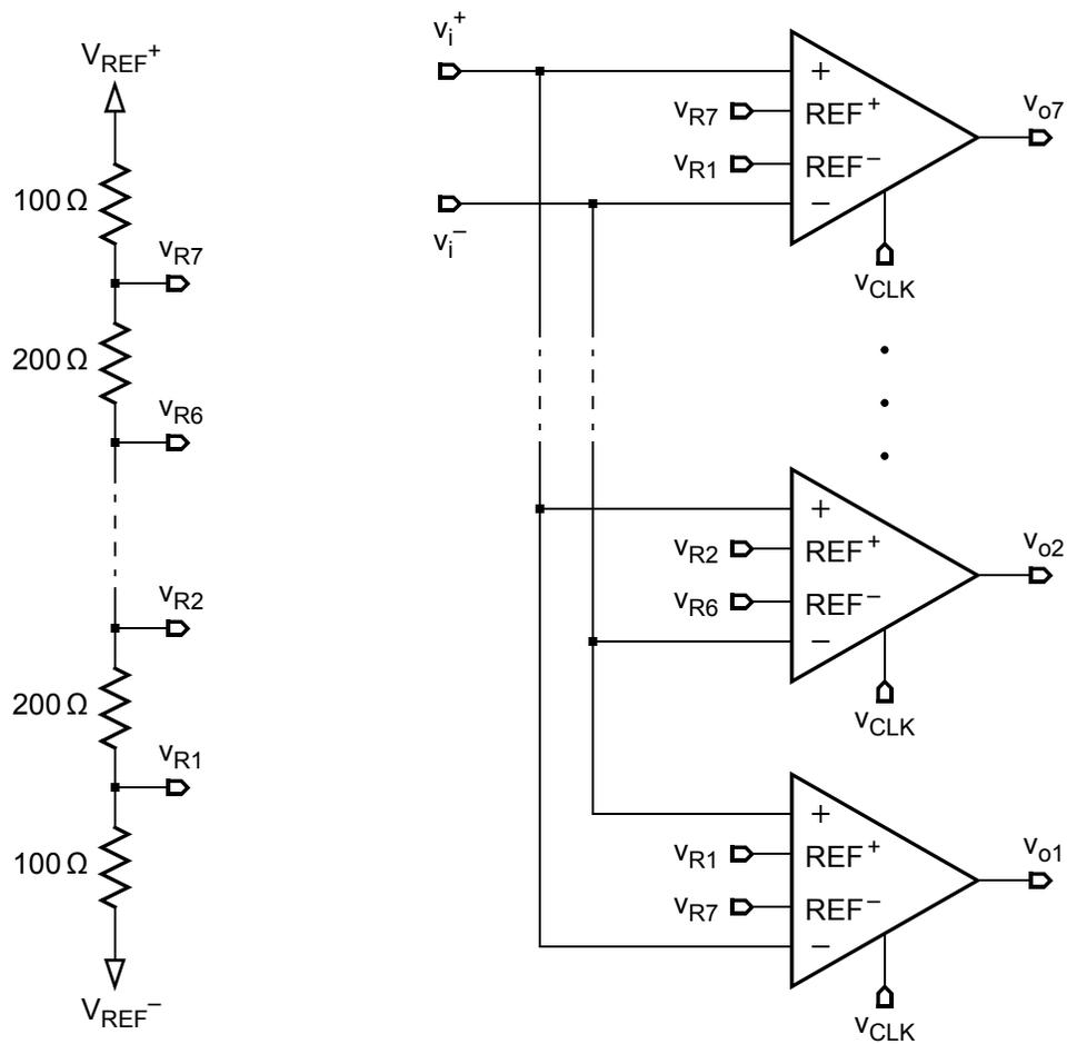
Figure 7.10: Circuit diagram of the flash ADC.
