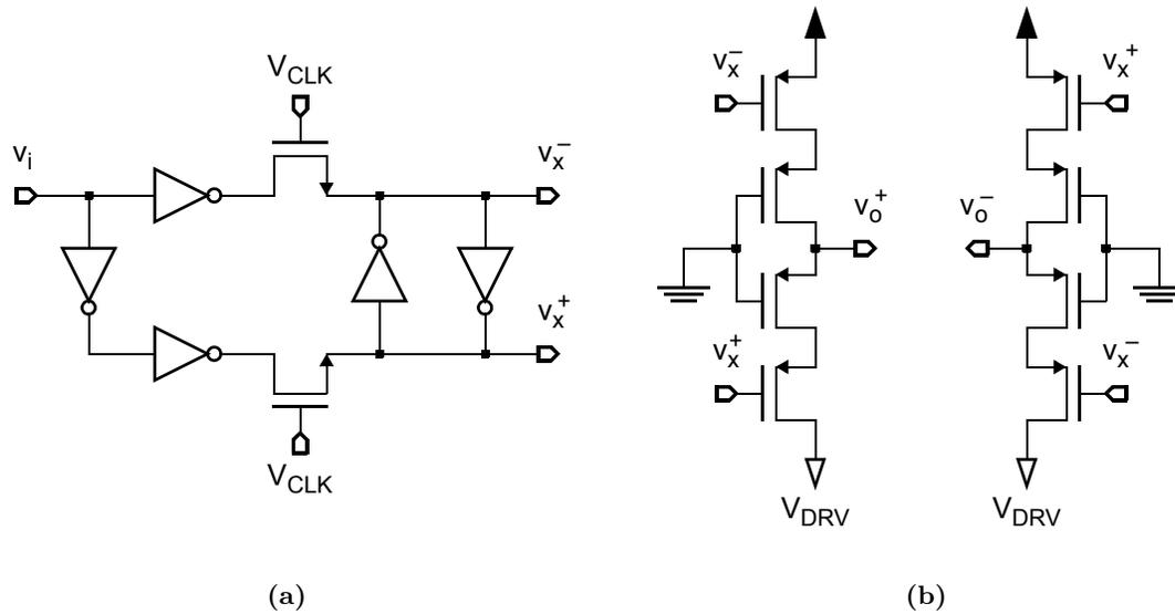
**Figure 7.14:** Circuit diagrams for: (a) the latch, and (b) the driver that are used prior to each unit element of the feedback DACs.
