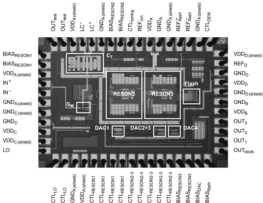
**Figure 8.1:** Chip micrograph of the experimental  $\Delta\Sigma$  modulator.
