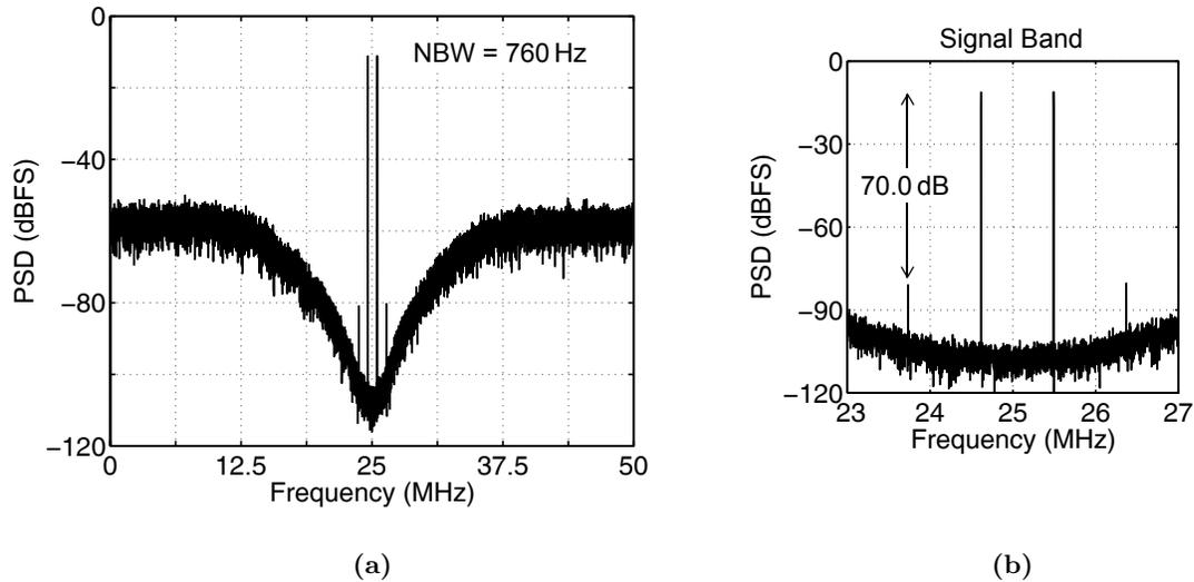
**Figure 6.11:** Simulated output spectrum of the experimental  $\Delta\Sigma$  modulator for two  $-11$  dBFS tones separated by 880 kHz: (a) from 0 to  $f_S/2$ , and (b) over the signal band ( $f_{Co} - f_B/2$  to  $f_{Co} + f_B/2$ ). This plot demonstrates the effect of non-linear distortion, as compared to Figure 6.10.
