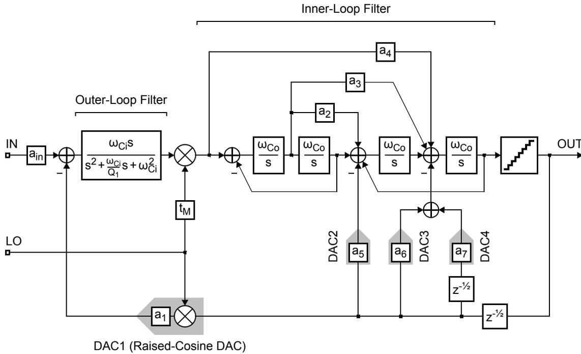
Figure 6.3: Complete block diagram for the experimental  $\Delta\Sigma$  modulator.
