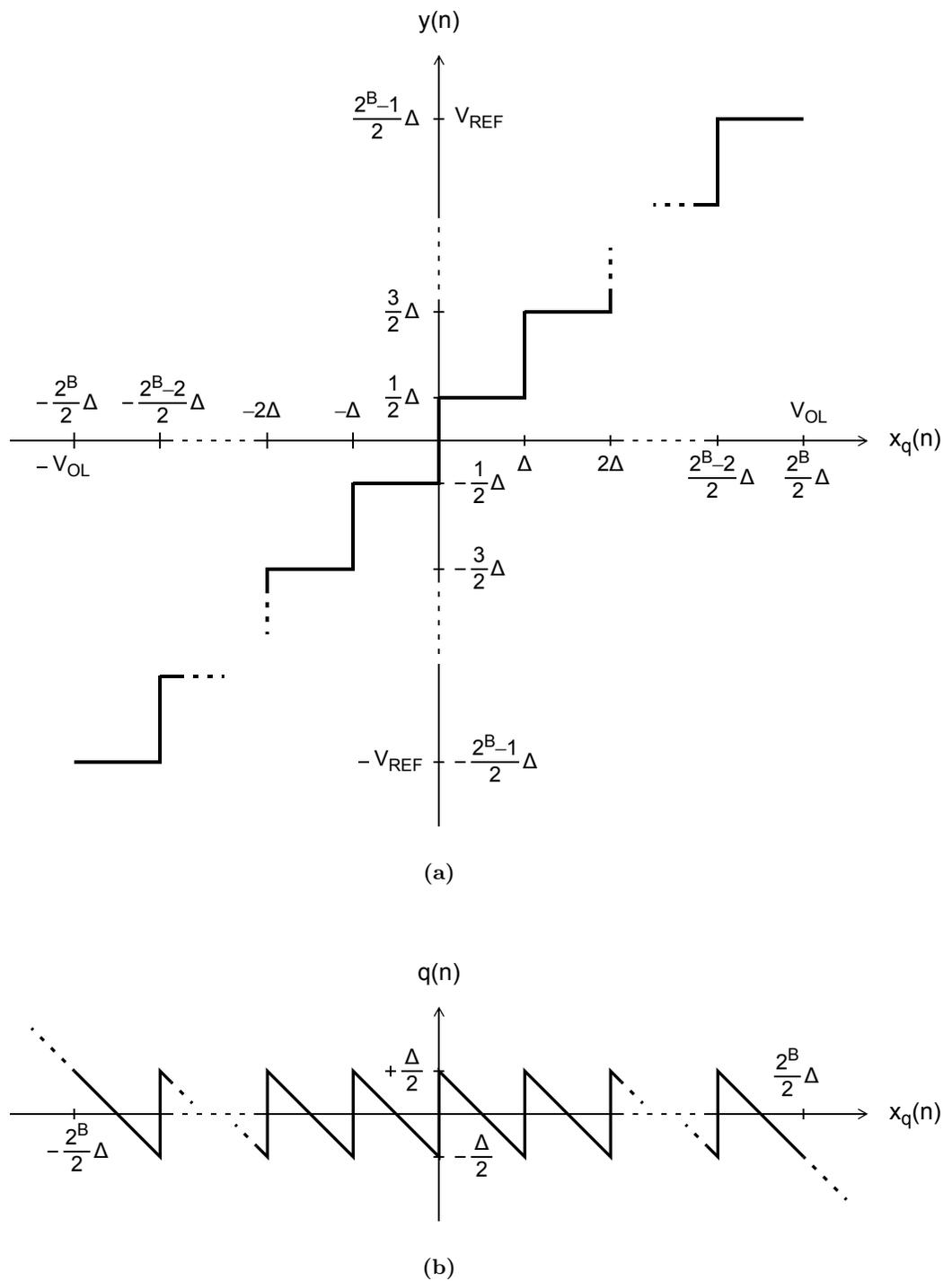
**Figure 2.1:** (a) The transfer characteristic of a uniform mid-rise quantizer that is designed with  $B$  quantization bits [Ham04], and (b) its associated quantization error.
