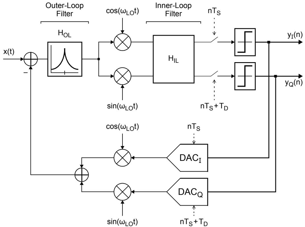
**Figure 2.14:** Block diagram for an image-reject frequency-translating  $\Delta\Sigma$  modulator.
