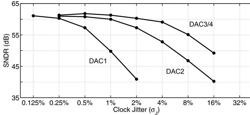
**Figure 6.12:** Simulated SNDR of the experimental  $\Delta\Sigma$  modulator as a function of the clock jitter introduced at each of its feedback DACs (DAC1–DAC4).
