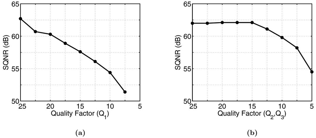
**Figure 6.13:** Simulated SQNR of the experimental  $\Delta\Sigma$  modulator as a function of: (a) the quality factor ( $Q_1$ ) of its LC resonator, and (b) the quality factors ( $Q_2, Q_3$ ) of its active-RC resonators.
