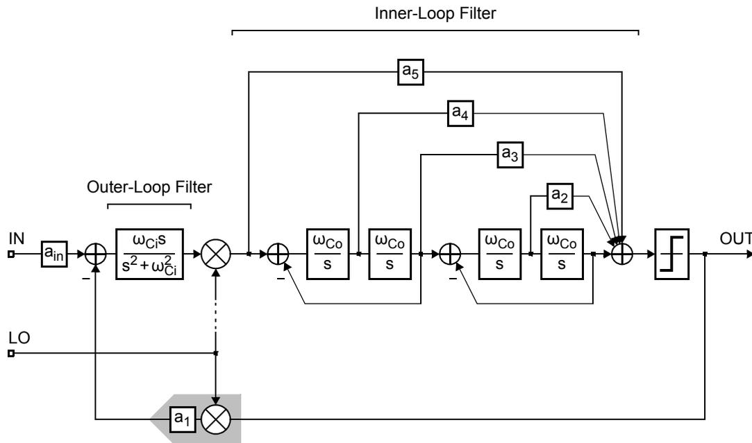
**Figure 5.10:** Block diagram for a 6th-order single-path frequency-translating  $\Delta\Sigma$  modulator that is designed with a strictly-feedforward loop-filter topology.
