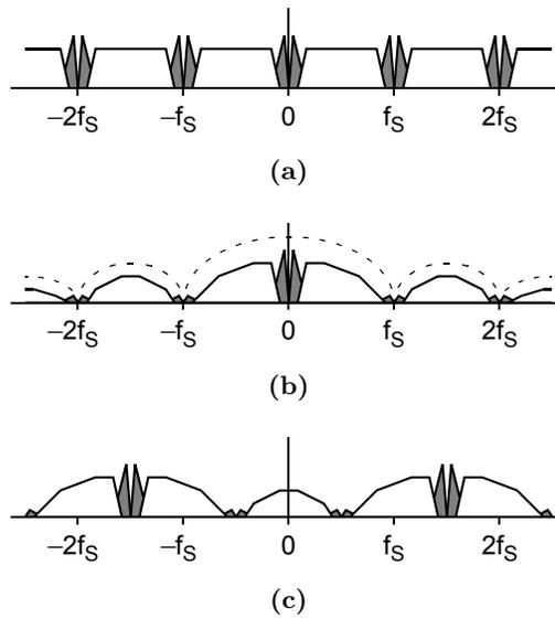
**Figure 5.7:** Frequency spectrum over the feedback path of a single-path frequency-translating  $\Delta\Sigma$  modulator with a *lowpass* inner-loop filter: (a) at the output of the  $\Delta\Sigma$  modulator  $y(n)$ , (b) after the feedback DAC  $y(t)$ , and (c) after the upconversion mixer  $x_1(t)$ . In this figure,  $f_{LO}$  is set to  $3f_s/2$ .
