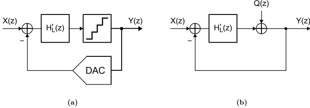
**Figure 2.6:** Block diagrams for: (a) a  $\Delta\Sigma$  modulator, and (b) its linear model.
