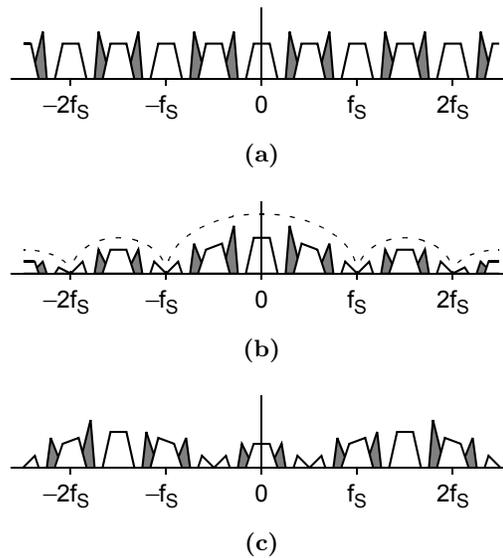
**Figure 5.8:** Frequency spectrum over the feedback path of a single-path frequency-translating  $\Delta\Sigma$  modulator with a *bandpass* inner-loop filter: (a) at the output of the  $\Delta\Sigma$  modulator  $y(n)$ , (b) after the feedback DAC  $y(t)$ , and (c) after the upconversion mixer  $x_1(t)$ . In this figure,  $f_{LO}$  is set to  $3f_s/2$ .
