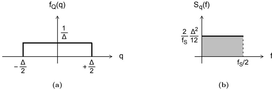
**Figure 2.2:** (a) The probability density function of the quantization error, and (b) its single-sided power spectral density under the additive white noise approximation.
