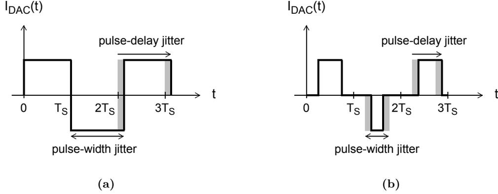
**Figure 3.4:** The effect of pulse-width and pulse-delay jitter on: (a) a non-return-to-zero (NRZ) pulse, and (b) a return-to-zero (RZ) pulse.
