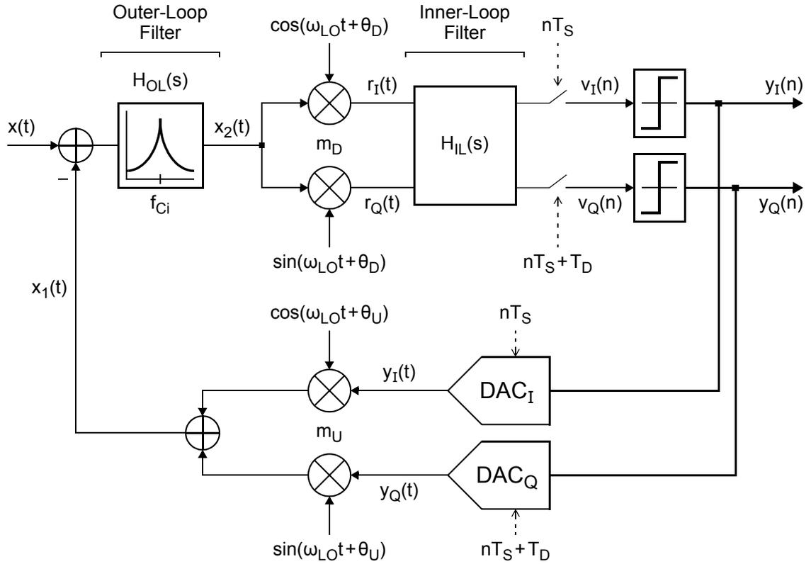
**Figure 4.1:** Block diagram for an image-reject frequency-translating  $\Delta\Sigma$  modulator. Here,  $T_S$  is the sampling period, and  $T_D$  is the quadrature-path sampling delay.
