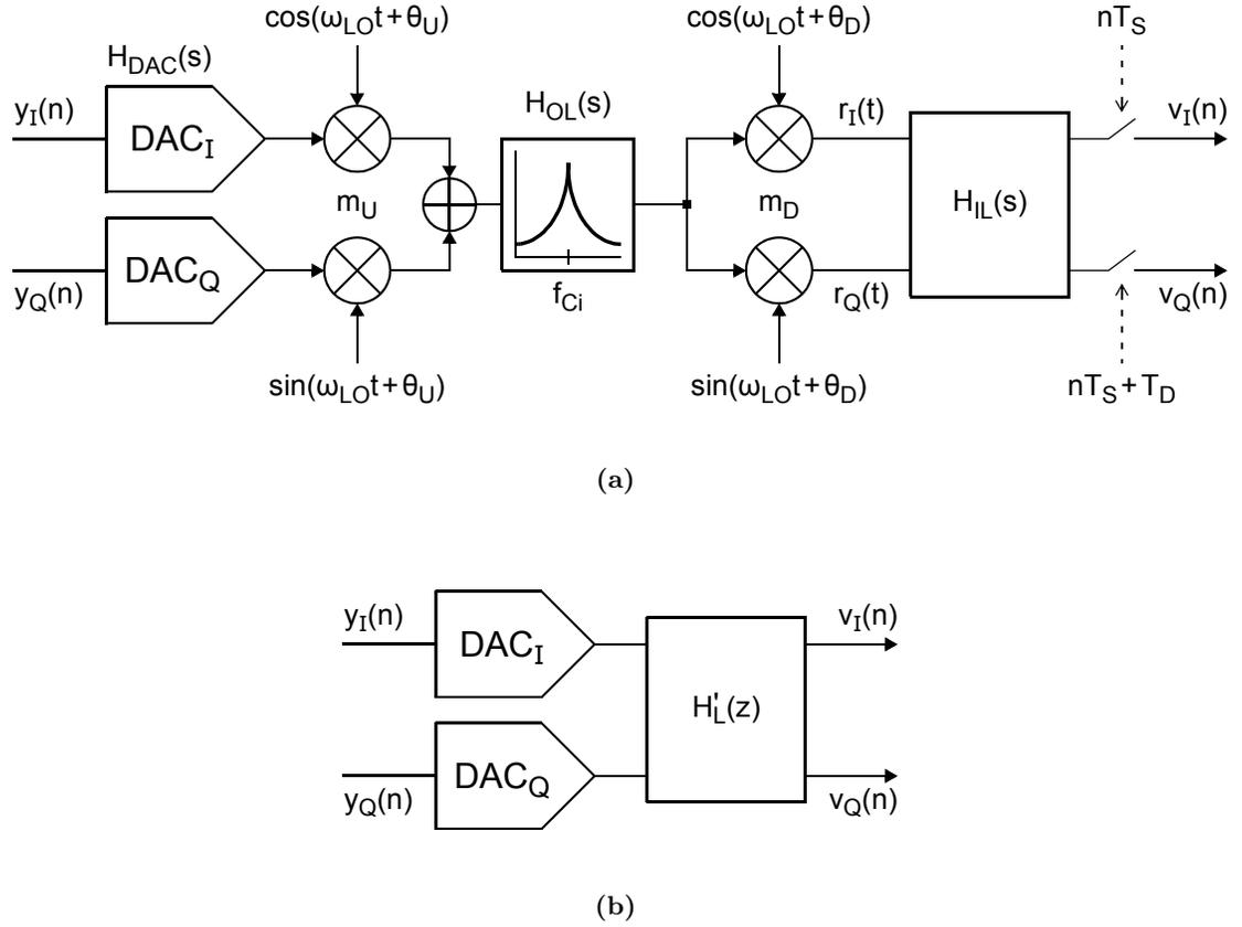
**Figure 4.3:** The loop feedback paths of: (a) the image-reject frequency-translating  $\Delta\Sigma$  modulator in Figure 4.1, and (b) the equivalent discrete-time complex  $\Delta\Sigma$  modulator in Figure 4.2.
