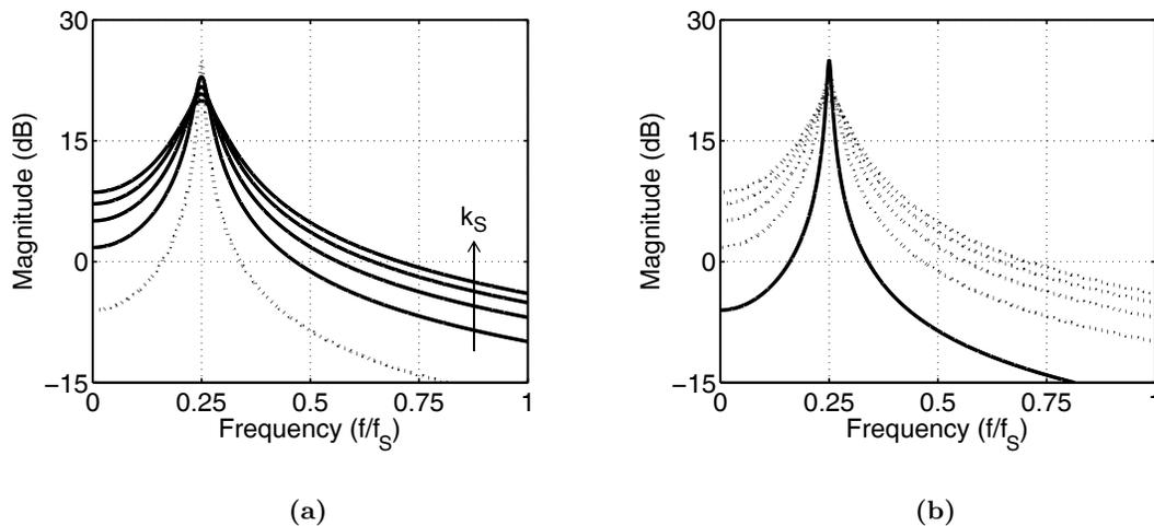
**Figure 5.12:** (a) The effective filtering characteristic of the outer-loop path  $\hat{H}_{OL}(s)$  of a single-path frequency-translating  $\Delta\Sigma$  modulator (Section 5.3), where  $k_S$  is varied from 1 to 4, and (b) the filtering characteristic of one resonator in a conventional bandpass  $\Delta\Sigma$  modulator.
