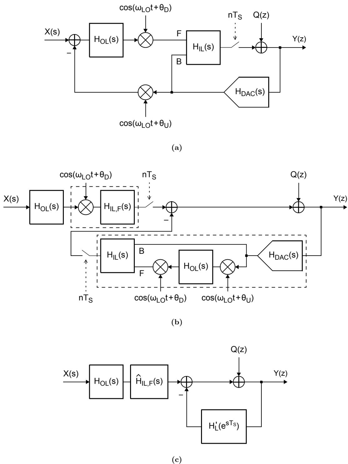
**Figure 5.18:** (a) The linear model of a single-path frequency-translating  $\Delta\Sigma$  modulator, (b) the  $\Delta\Sigma$  modulator in (a), modified so that the forward component of its inner-loop filter  $H_{IL,F}(s)$  is separated from  $H_{IL}(s)$ , and (c) the model that is used to derive the effective STF.
