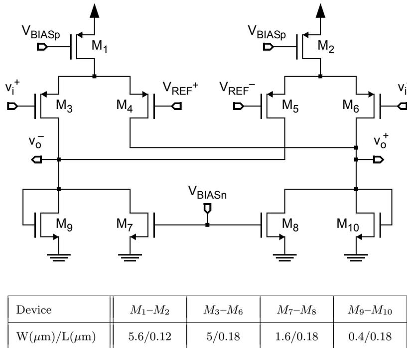
**Figure 7.11:** Circuit diagram of the pre-amplifier.
