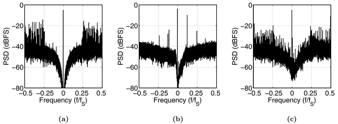
**Figure 4.9:** The output spectrum of the test architecture shown in Figure 4.8, when it is designed with: (a)  $T_S = 3T_{LO}/2$  and  $T_D = T_S/2$ , (b)  $T_S = 3.125T_{LO}/2$  and  $T_D = T_S/2$ , and (c)  $T_S = 3.5T_{LO}/2$  and  $T_D = T_S/2$ . Here, the configuration in (a) satisfies the constraints in Equations (4.12) and (4.13), whereas those in (b) and (c) violate the constraint in Equation (4.12).
