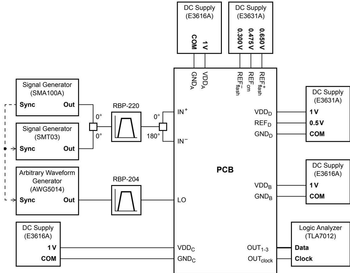
**Figure 8.3:** Test setup of the experimental prototype for a two-tone input signal.
