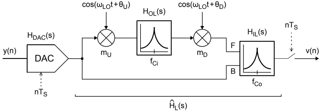
**Figure 5.15:** The loop feedback path of a single-path frequency-translating  $\Delta\Sigma$  modulator that is designed with a hybrid feedforward-feedback loop-filter topology.
