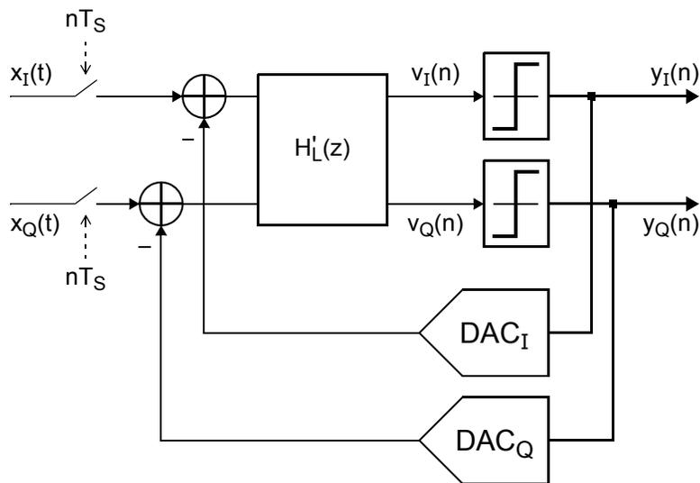
**Figure 4.2:** Block diagram for a discrete-time  $\Delta\Sigma$  modulator with a complex loop filter.
