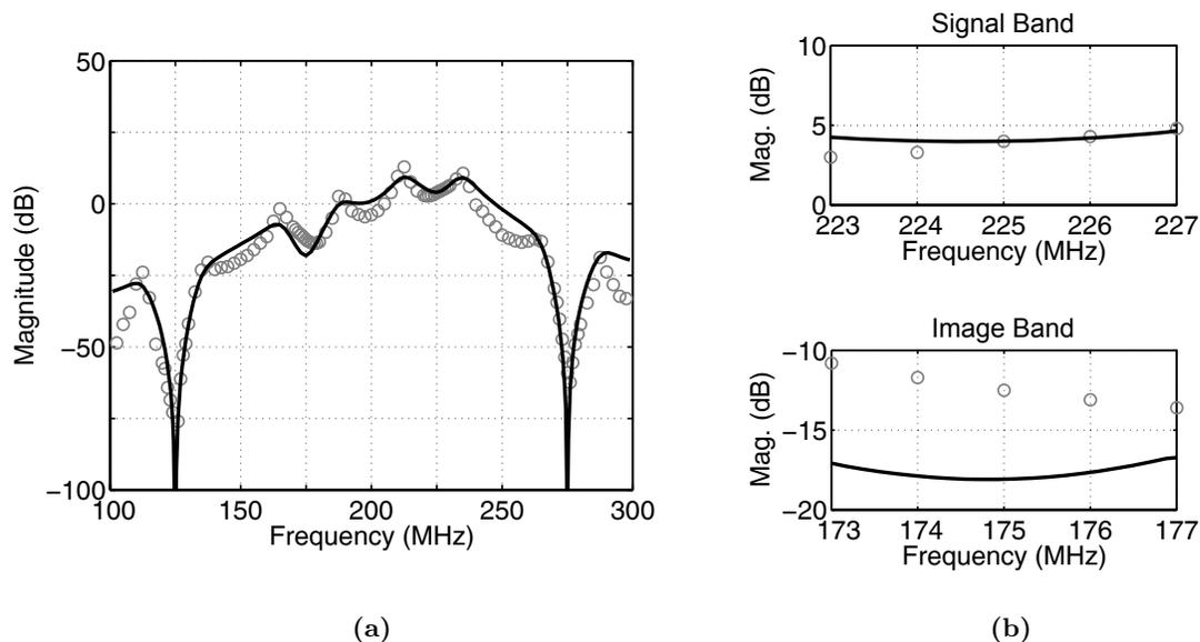
**Figure 8.9:** The measured STF of the experimental  $\Delta\Sigma$  modulator: (a) from  $f_S$  to  $3f_S$ , (b) over the signal band and over the image band. Here, — denotes simulation results (Figure 6.7), and  $\circ$  denotes measurement results.
