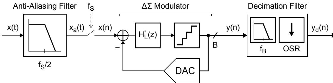
**Figure 2.8:** Block diagram for a  $\Delta\Sigma$  ADC.
