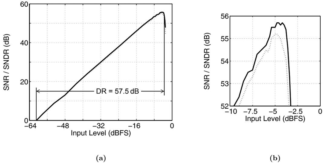
**Figure 8.5:** Measured SNR and SNDR of the experimental  $\Delta\Sigma$  modulator as a function of its input level for an input tone at 224.6 MHz. (SNR — and SNDR  $\cdots$ )
