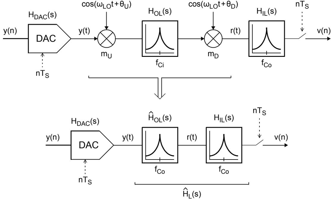
**Figure 5.5:** The *effective* loop feedback path of the single-path frequency-translating  $\Delta\Sigma$  modulator in Figure 5.1, which combines the upconversion and downconversion operations with the response of the outer-loop filter  $H_{OL}(s)$ .
