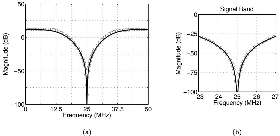
**Figure 6.6:** The simulated NTF of the experimental  $\Delta\Sigma$  modulator (Figure 6.3): (a) from 0 to  $f_S/2$ , and (b) over the signal band ( $f_{Co} - f_B/2$  to  $f_{Co} + f_B/2$ ). In this figure,  $\circ$  denotes results derived from behavioural simulations, and  $—$  denotes results derived from equations.
