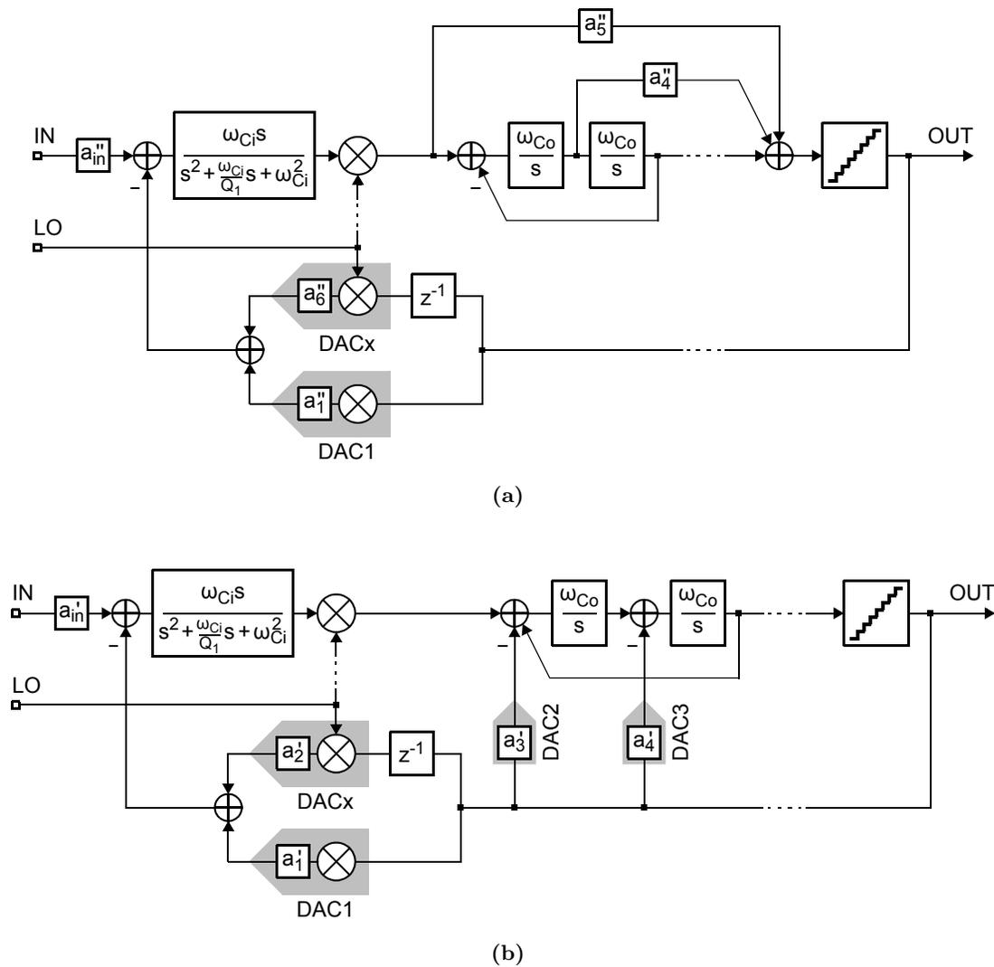
**Figure 6.4:** Block diagrams for: (a) a strictly-feedforward, and (b) a strictly-feedback configuration of the  $\Delta\Sigma$  modulator in Figure 6.3, showing the additional required coefficient path ( $DACx$ ).
