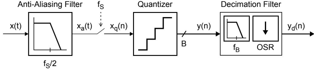
**Figure 2.5:** Block diagram for an oversampling ADC.
