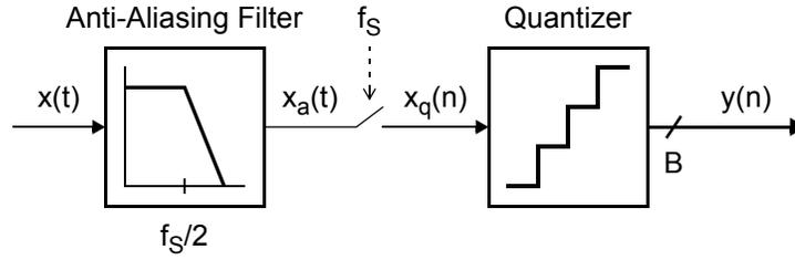
**Figure 2.3:** Block diagram for a Nyquist-rate ADC.
