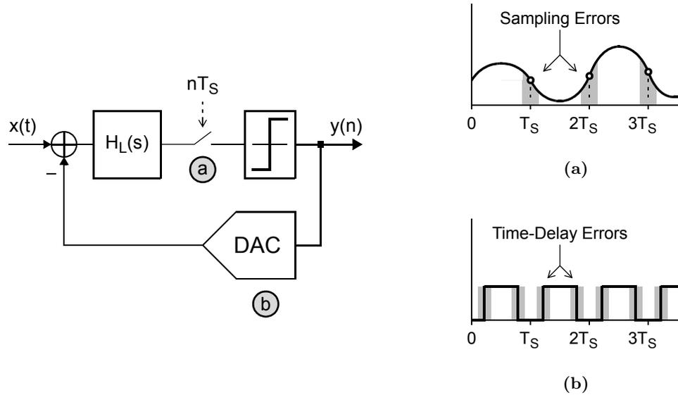
**Figure 3.3:** Timing errors in a continuous-time  $\Delta\Sigma$  modulator: (a) sampling errors in the forward path, and (b) time-delay errors in the feedback DAC.
