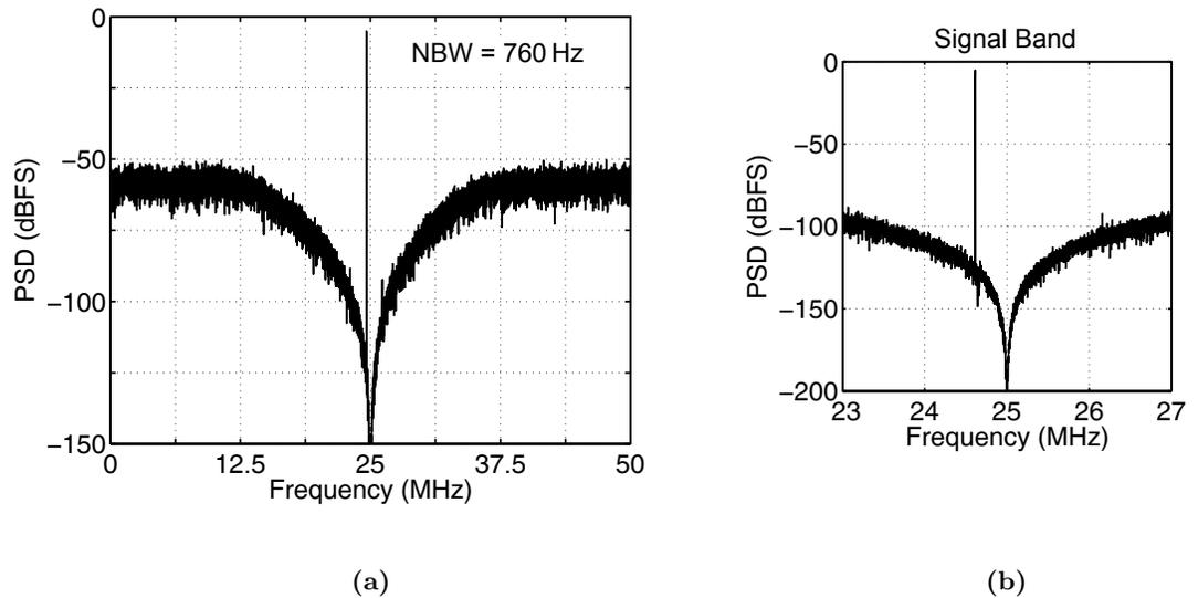
**Figure 6.9:** Simulated output spectrum of the experimental  $\Delta\Sigma$  modulator for a  $-5$  dBFS input tone at 224.6 MHz: (a) from 0 to  $f_S/2$ , and (b) over the signal band ( $f_{Co} - f_B/2$  to  $f_{Co} + f_B/2$ ).
