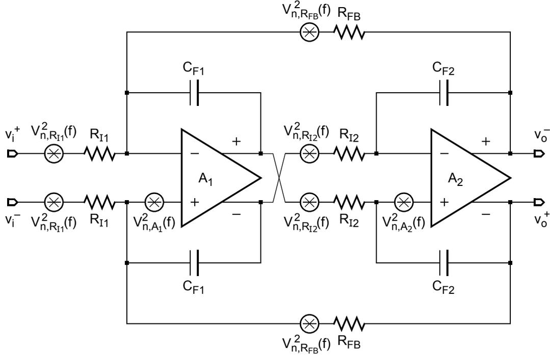
**Figure 7.7:** Sources of thermal noise in the active-RC resonators.
