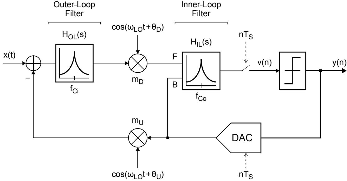
**Figure 5.14:** General block diagram for a single-path frequency-translating  $\Delta\Sigma$  modulator that has a hybrid feedforward-feedback loop-filter topology.
