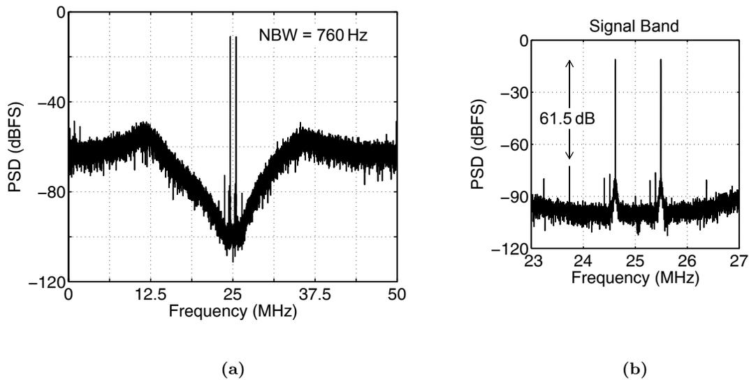
**Figure 8.7:** Measured output spectrum of the experimental  $\Delta\Sigma$  modulator for two  $-11$  dBFS tones separated by 880 kHz: (a) from 0 to  $f_S/2$ , and (b) over the signal band.
