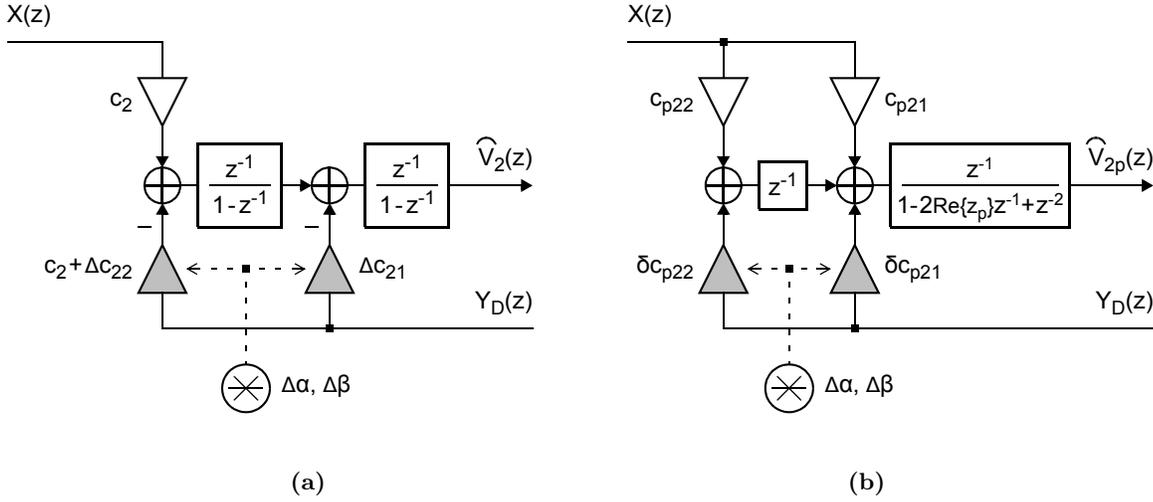
**Figure 3.8:** Realizations of: (a)  $\widehat{H}'_{L,2}(z)$  in Table 3.1, and (b)  $\widehat{H}'_{L,2p}(z)$  in Table 3.2. The terminal names in this figure correspond to the discrete-time  $\Delta\Sigma$  modulator in Figure 3.7.
