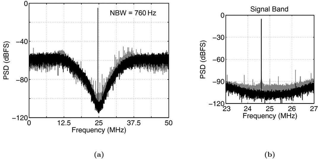
**Figure 8.8:** The simulated and measured output spectrum of the experimental  $\Delta\Sigma$  modulator for a  $-5$  dBFS input tone at 224.6 MHz: (a) from 0 to  $f_S/2$ , and (b) in the signal band. Here, the black spectrum denotes simulation results, and the grey spectrum denotes measurement results.
