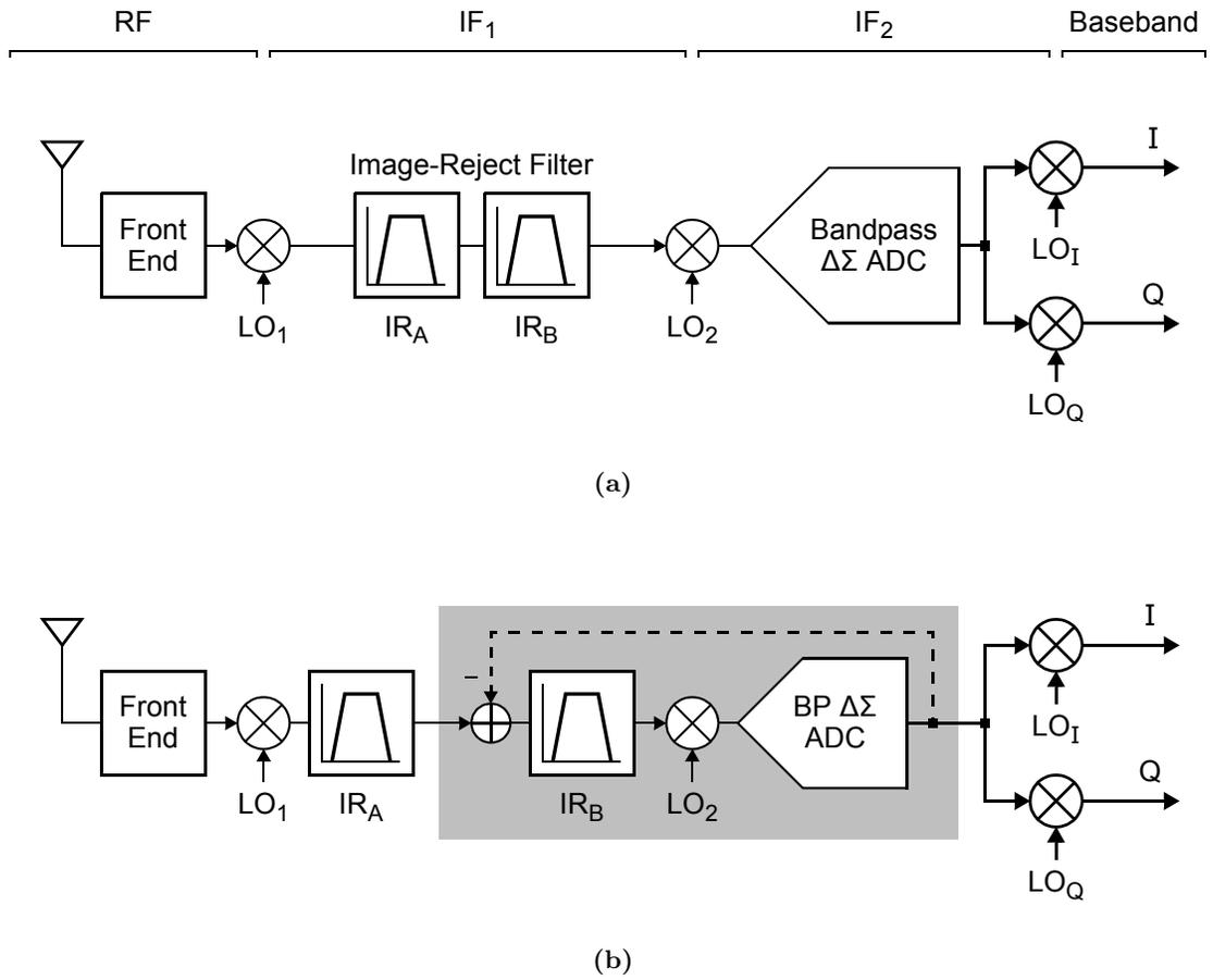
**Figure 1.1:** Block diagrams for: (a) a conventional digital-IF receiver, and (b) a digital-IF receiver that is based on the frequency-translating  $\Delta\Sigma$  ADC proposed in this thesis.
