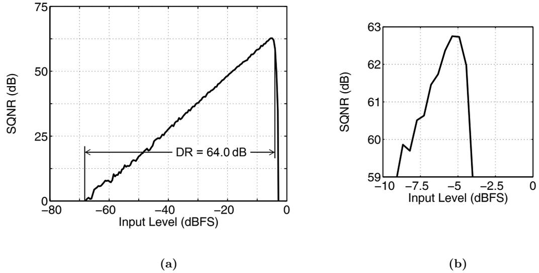
**Figure 6.8:** Simulated SQNR of the experimental  $\Delta\Sigma$  modulator, as a function of its input level, for an input tone at 224.6 MHz.
