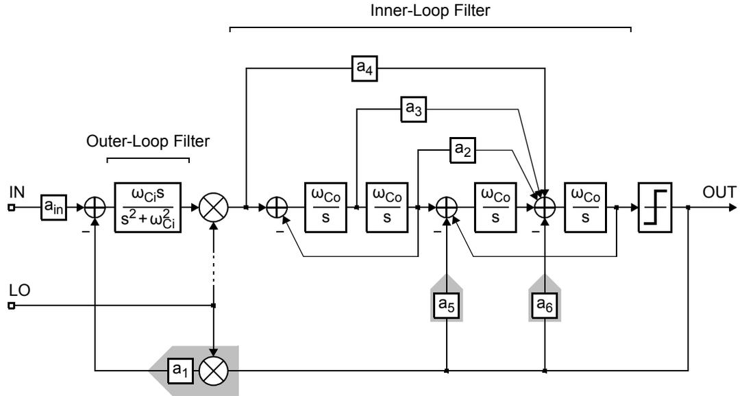
**Figure 5.13:** Block diagram for a 6th-order single-path frequency-translating  $\Delta\Sigma$  modulator that is designed with a hybrid feedforward-feedback loop-filter topology.
