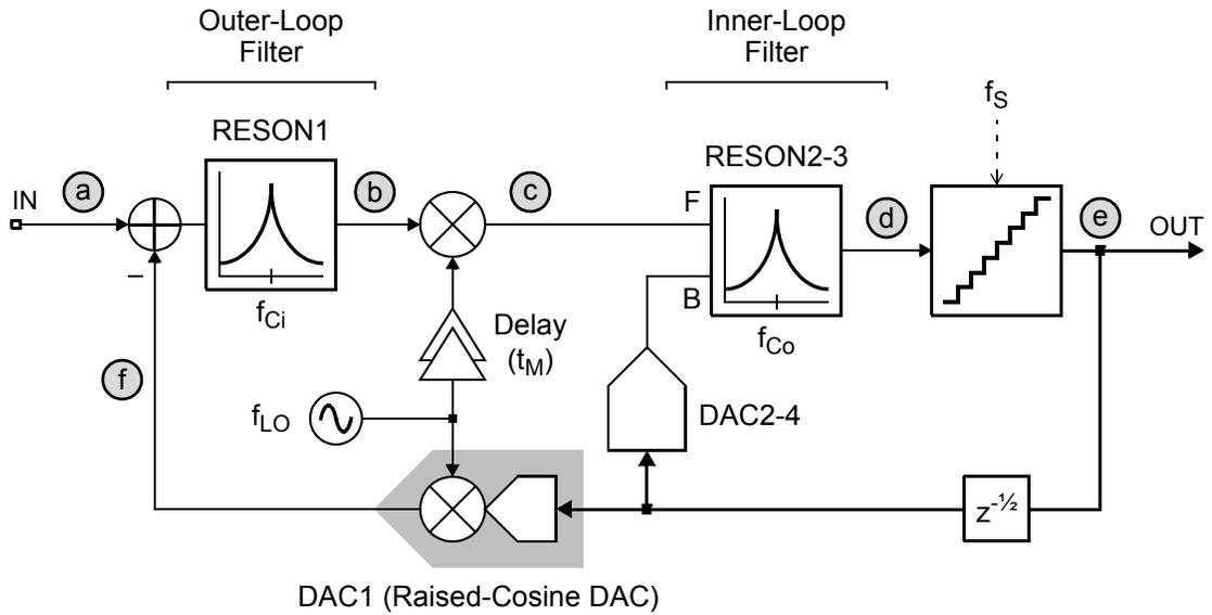
**Figure 6.1:** Simplified block diagram for the experimental  $\Delta\Sigma$  modulator.
