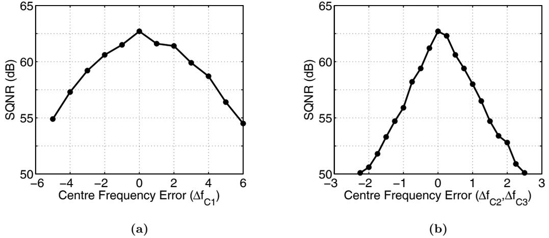
**Figure 6.14:** Simulated SQNR of the experimental  $\Delta\Sigma$  modulator as a function of: **(a)** the centre-frequency error ( $\Delta f_{C1}$ ) of its LC resonator, and **(b)** the centre-frequency errors ( $\Delta f_{C2}, \Delta f_{C3}$ ) of its active-RC resonators.
