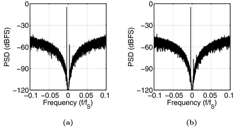
**Figure 4.14:** The output spectrum of the test architecture shown in Figure 4.8, when it is designed with  $T_S = 3T_{LO}/2$  and  $T_D = T_S/2$ . Here, an amplitude error of 0.5% is introduced into the LO signal that is applied to the quadrature mixer of: (a) the feedback path, and (b) the forward path.
