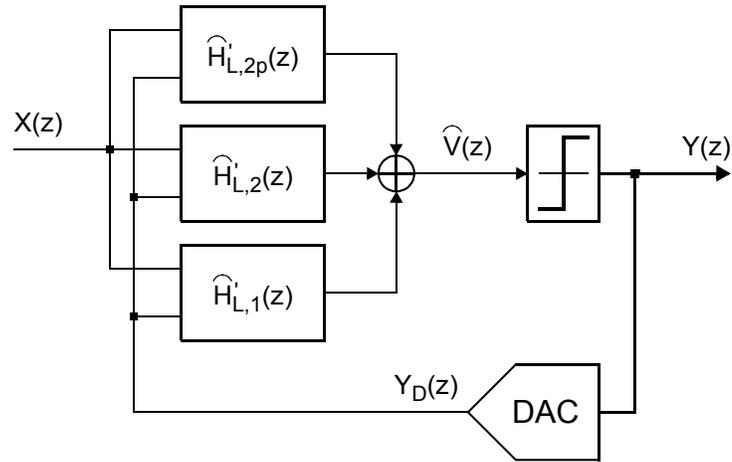
**Figure 3.7:** Block diagram for a discrete-time  $\Delta\Sigma$  modulator that is realized using the error-mapping terms in Tables 3.1 and 3.2.
