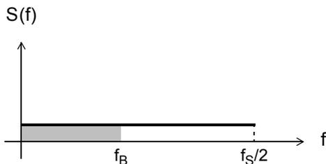
**Figure 2.4:** Power spectral density of the quantization error in an oversampling ADC.
