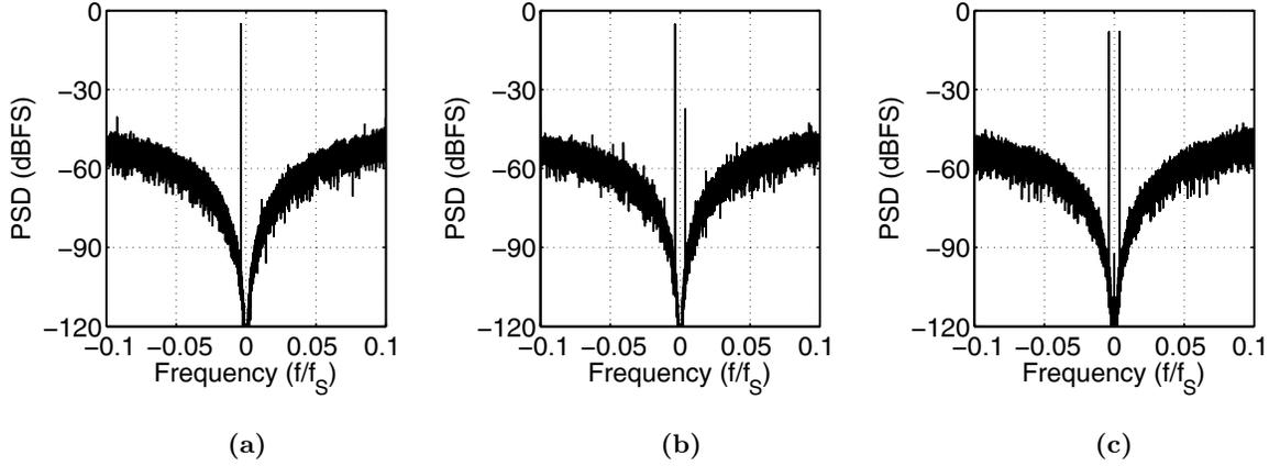
**Figure 4.10:** The output spectrum of the test architecture shown in Figure 4.8, when it is designed with: (a)  $T_S = 3T_{LO}/2$  and  $T_D = T_S/2$ , (b)  $T_S = 3T_{LO}/2$  and  $T_D = 0.95T_S/2$ , and (c)  $T_S = 3T_{LO}/2$  and  $T_D = 0$ . Here, the configuration in (a) satisfies the constraints in Equations (4.12) and (4.13), whereas those in (b) and (c) violate the constraint in Equation (4.13).
