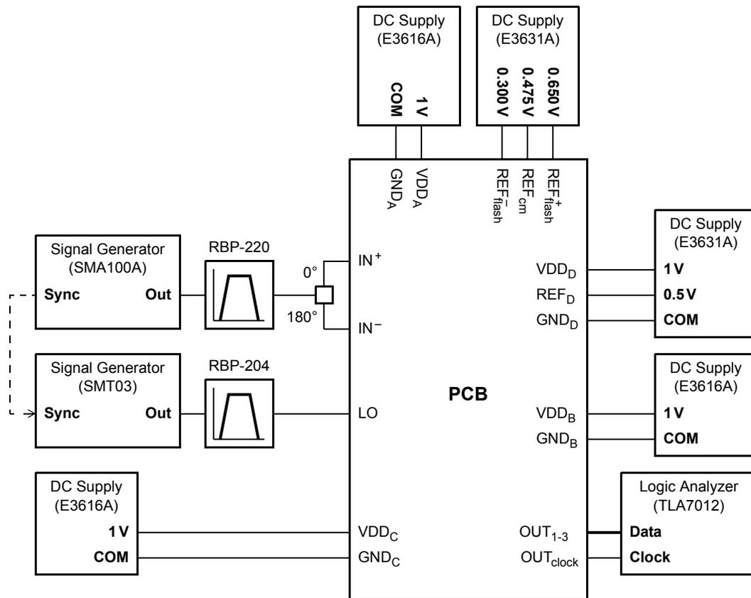
**Figure 8.2:** Test setup of the experimental prototype for a single-tone input signal.
