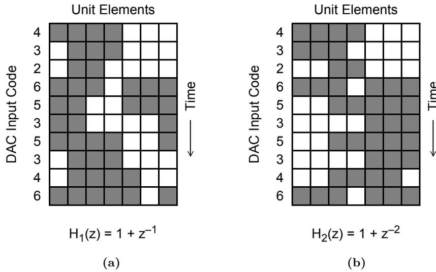
Figure 7.16: Element selection patterns for: (a)  $H_1(z)$ , and (b)  $H_2(z)$  [Shu98].
