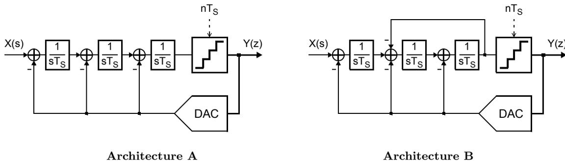
**Figure 3.10:** Block diagrams for the continuous-time  $\Delta\Sigma$  modulator architectures in Table 3.4.
