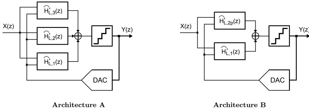
**Figure 3.11:** Block diagrams for discrete-time  $\Delta\Sigma$  modulators that use the error-mapping terms in Tables 3.1 and 3.2 to realize loop transfer functions that are equivalent to those in Table 3.4.
