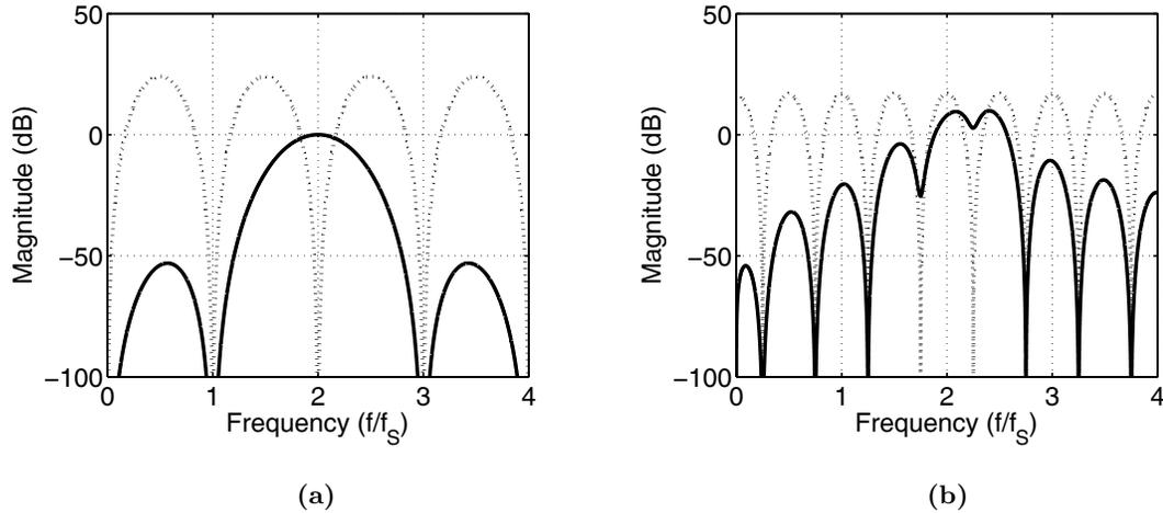
**Figure 5.2:** Simulated STF and NTF of: **(a)** an image-reject frequency-translating  $\Delta\Sigma$  modulator with  $f_{Ci} = 2f_S$ , and **(b)** a single-path frequency-translating  $\Delta\Sigma$  modulator with  $f_{Ci} = 9/4f_S$ . Here, the image band of the single-path architecture is centred at  $7/4f_S$ . (STF — and NTF  $\cdots$ )
