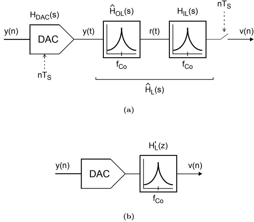
**Figure 5.6:** The *effective* loop feedback path of a single-path frequency-translating  $\Delta\Sigma$  modulator, and the loop feedback path of a discrete-time bandpass  $\Delta\Sigma$  modulator.
