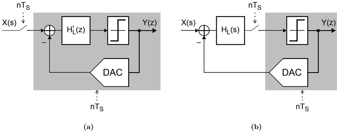
**Figure 2.9:** Block diagrams for: (a) a discrete-time  $\Delta\Sigma$  modulator, and (b) a continuous-time  $\Delta\Sigma$  modulator. Here,  $T_s$  represents the sampling period.
