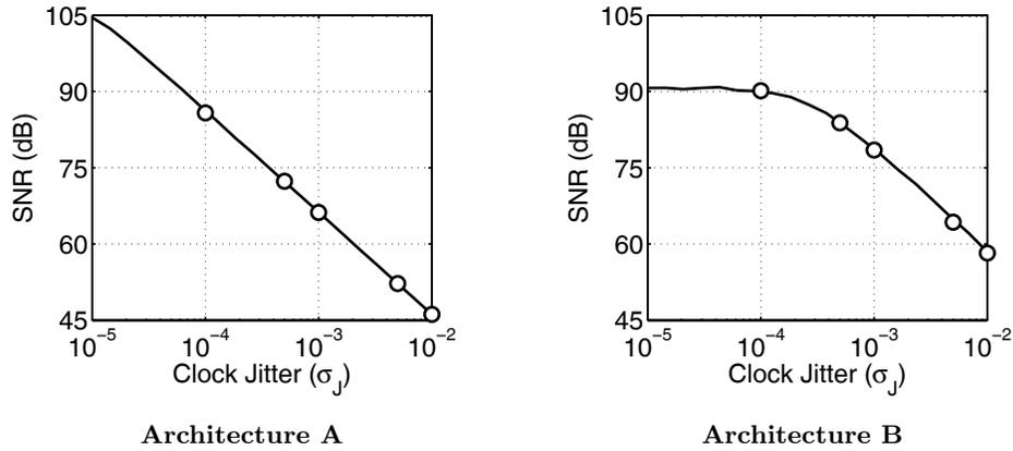
**Figure 3.12:** The simulated SNR, as a function of the normalized clock jitter, for Architectures A and B specified in Table 3.4. Here, — denotes results derived from the presented modeling technique, and  $\circ$  denotes results derived from the Simulink behavioural model.
