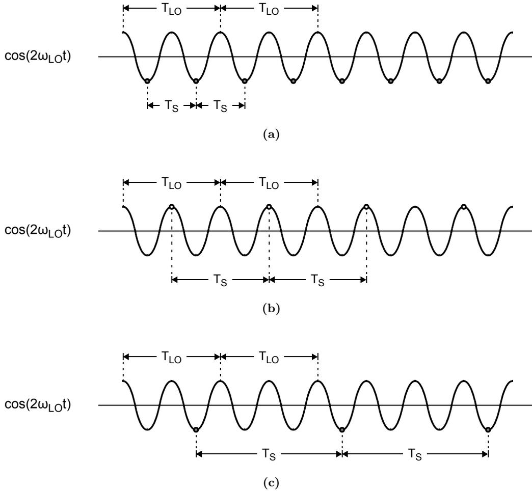
**Figure 4.4:** Timing of the quadrature-path sampling instants ( $t_{nd}$ ) for  $T_D = T_S/2$ .
