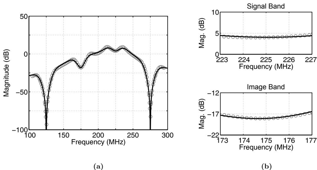
**Figure 6.7:** The simulated STF of the experimental  $\Delta\Sigma$  modulator (Figure 6.3): (a) from  $f_s$  to  $3f_s$ , (b) over the signal band ( $f_{Ci} - f_B/2$  to  $f_{Ci} + f_B/2$ ) and over the image band. Here,  $\circ$  denotes results derived from behavioural simulations, and  $—$  denotes results derived from equations.
