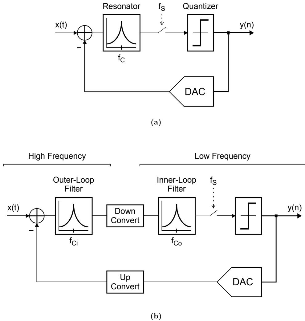
**Figure 2.12:** General block diagrams for bandpass  $\Delta\Sigma$  modulators: (a) a conventional architecture, and (b) a downconversion architecture.
