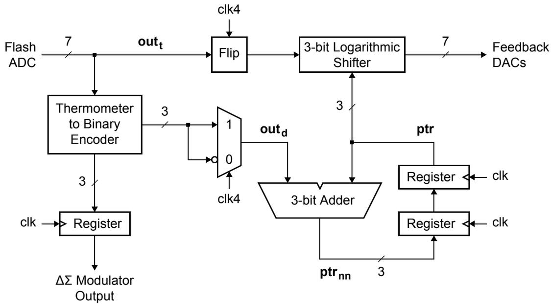
Figure 7.17: Block diagram for the bandpass mismatch-shaping logic.
