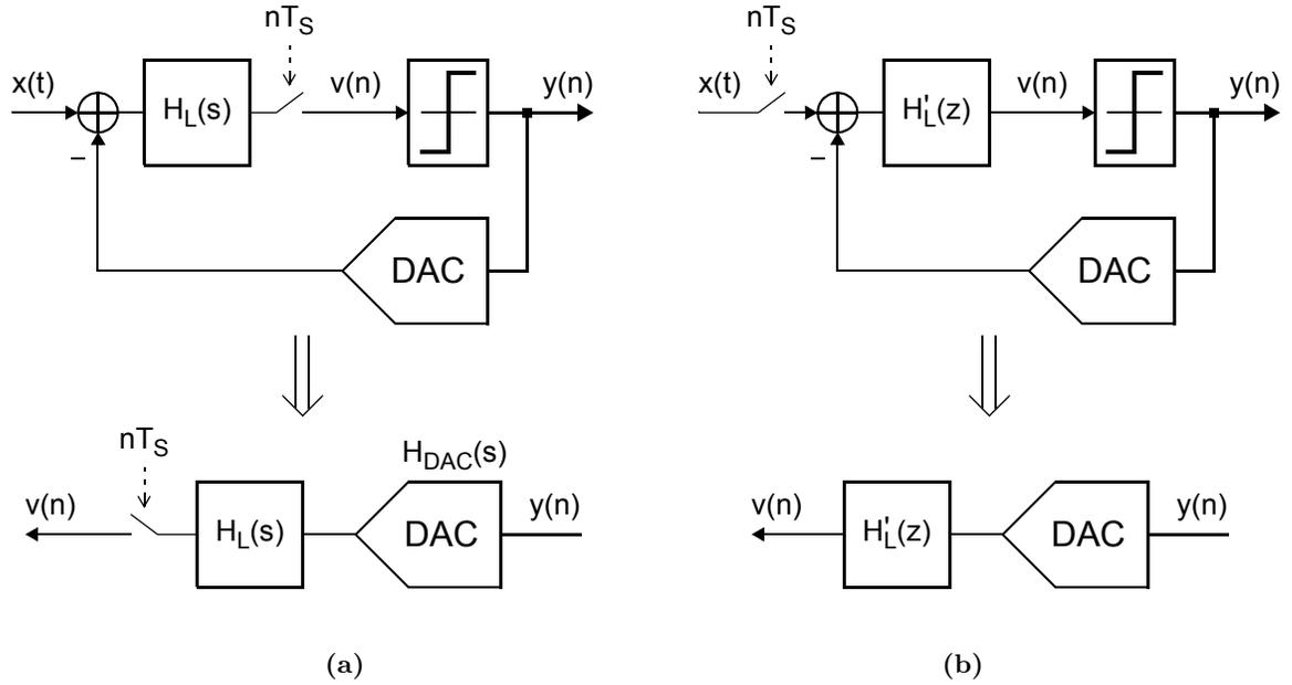
**Figure 3.1:** The loop feedback paths of: (a) a continuous-time  $\Delta\Sigma$  modulator, and (b) an equivalent discrete-time  $\Delta\Sigma$  modulator.
