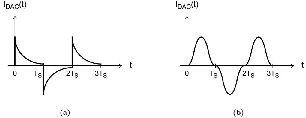
**Figure 3.5:** (a) An exponential DAC pulse, and (b) a raised-cosine DAC pulse.
