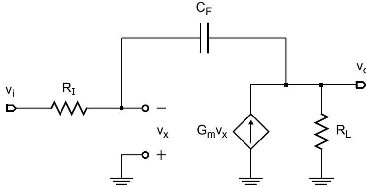
**Figure 7.6:** Circuit diagram of a standard active-RC integrator.
