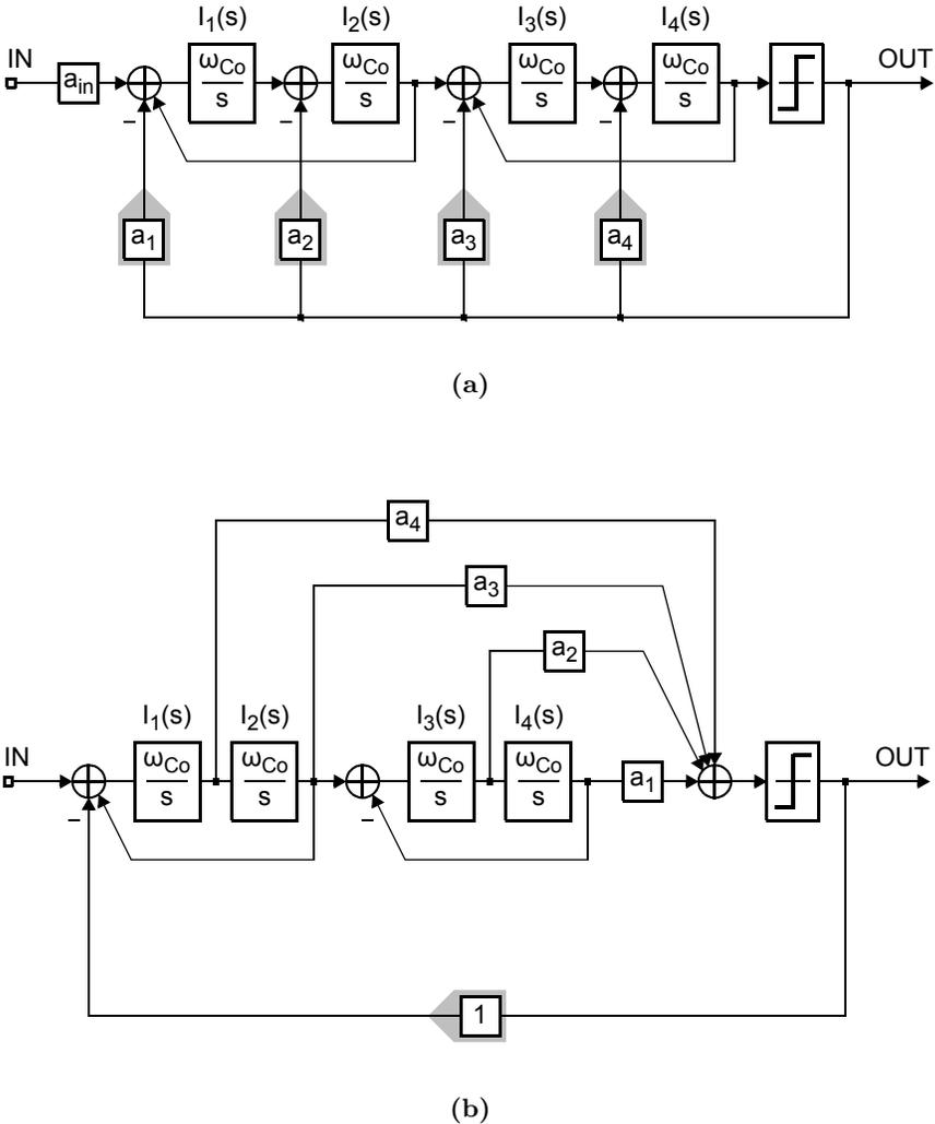
**Figure 5.11:** Block diagrams for a conventional 4th-order bandpass  $\Delta\Sigma$  modulator that is designed with: (a) a strictly-feedback loop-filter topology, and (b) a strictly-feedforward topology.
