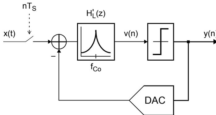
**Figure 5.3:** Block diagram for a discrete-time  $\Delta\Sigma$  modulator with a bandpass loop filter.
