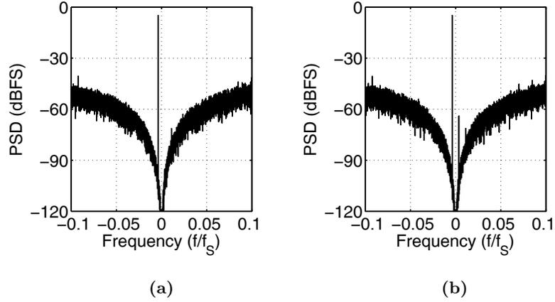
**Figure 4.13:** The output spectrum of the test architecture shown in Figure 4.8, when it is designed using  $T_S = 3T_{LO}/2$  and  $T_D = T_S/2$ . Here, a time-delay error of  $\Delta t$  is introduced into the response of the quadrature-path feedback DAC, where: (a)  $\Delta t = 0.0005T_S$ , and (b)  $\Delta t = 0.05T_S$ .
