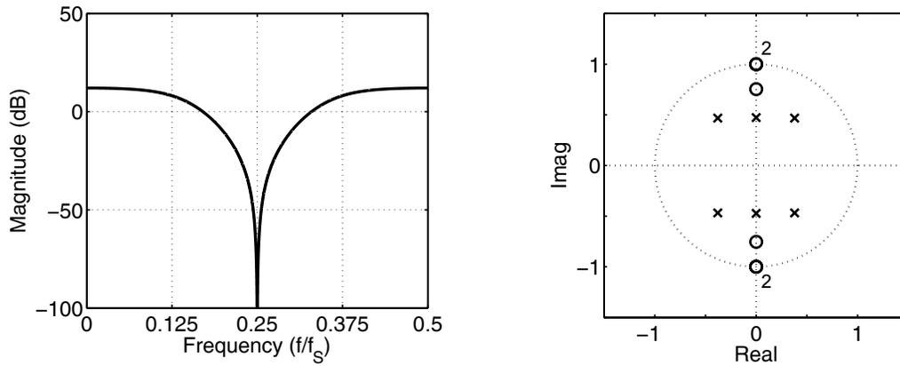
**Figure 6.5:** Magnitude response and pole-zero map of the prototype NTF.
