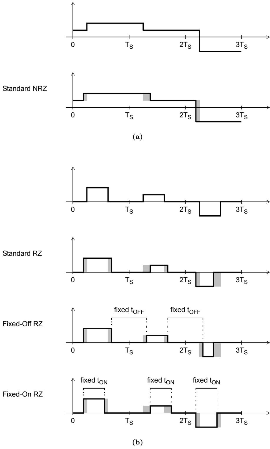
**Figure 3.14:** The rectangular DAC pulses that are studied in the analysis. (a) An NRZ pulse with ideal timing, and one affected by clock jitter. (b) An RZ pulse with ideal timing, and three affected by clock jitter. Here, the effect of timing errors is shown for RZ pulses with: standard timing, a fixed off-time duration, and a fixed on-time duration.
