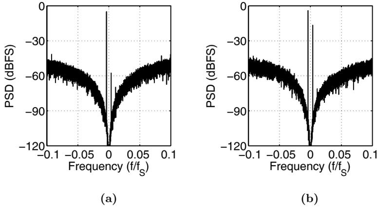
**Figure 4.11:** The output spectrum of the test architecture shown in Figure 4.8, when it is designed with  $T_S = 3T_{LO}/2$  and  $T_D = T_S/2$ . Here, a phase error of  $\Delta\theta$  is introduced into the LO signal that is applied to the quadrature mixer in the *feedback* path, where: (a)  $\Delta\theta = 0.0015\pi$ , and (b)  $\Delta\theta = 0.15\pi$ .
