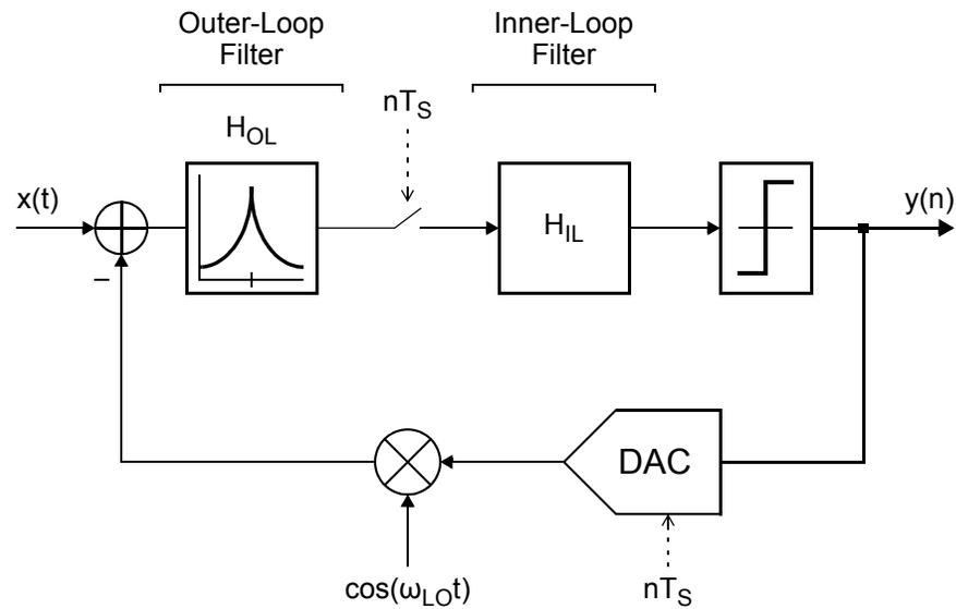
**Figure 2.13:** Block diagram for a subsampling  $\Delta\Sigma$  modulator.
