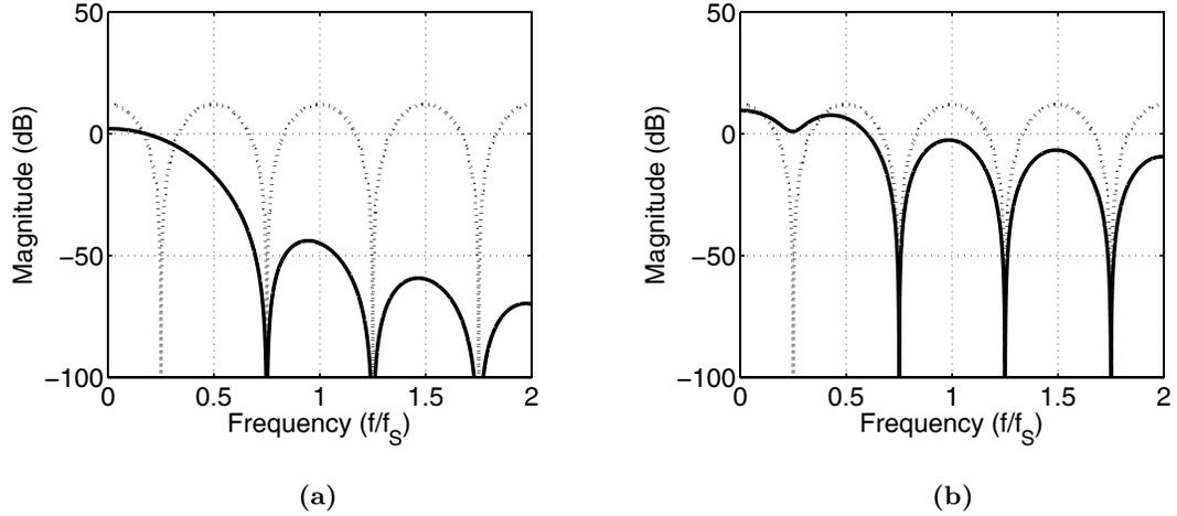
**Figure 2.11:** Simulated STF and NTF of a 4th-order bandpass  $\Delta\Sigma$  modulator with: **(a)** a feedback loop-filter topology, and **(b)** a feedforward loop-filter topology. Here, the signal band of the bandpass  $\Delta\Sigma$  modulator is centred at  $1/4f_s$ . (STF — and NTF  $\cdots$ )
