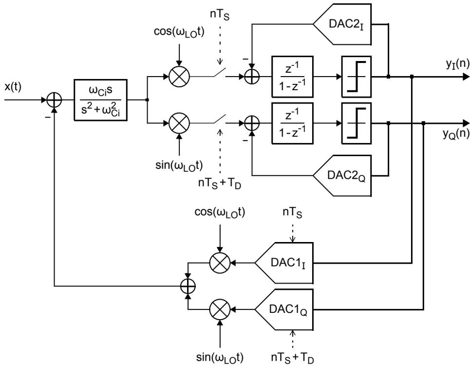
**Figure 4.8:** A test image-reject frequency-translating  $\Delta\Sigma$  modulator architecture.
