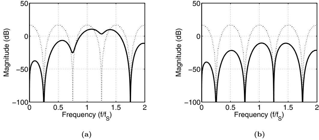
**Figure 5.19:** Simulated STF for the: (a) low-frequency term, and (b) high-frequency term of a single path frequency-translating  $\Delta\Sigma$  modulator with  $f_{Ci} = 5/4f_s$ . (STF — and NTF ···)
