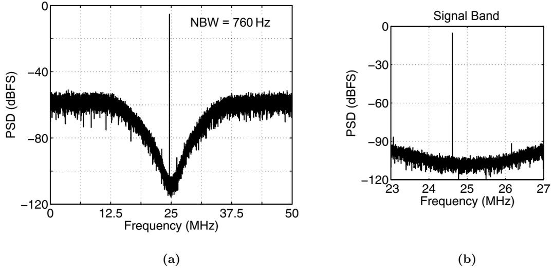
**Figure 6.10:** Simulated output spectrum of the experimental  $\Delta\Sigma$  modulator for a  $-5$  dBFS input tone at 224.6 MHz: (a) from 0 to  $f_S/2$ , and (b) over the signal band ( $f_{Co} - f_B/2$  to  $f_{Co} + f_B/2$ ). This plot demonstrates the effect of circuit noise, as compared to Figure 6.9.
