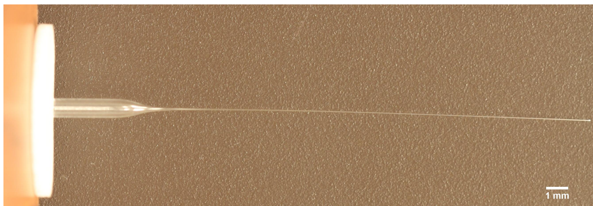
FIGURE 3.1: An X-ray diffraction tube is shown here. The diameter of the tube is 8mm at the left side, quickly tapered to mm size, then more slowly tapered 100 \mu\text{m} outer diameter with 10 \mu\text{m} thick walls.
