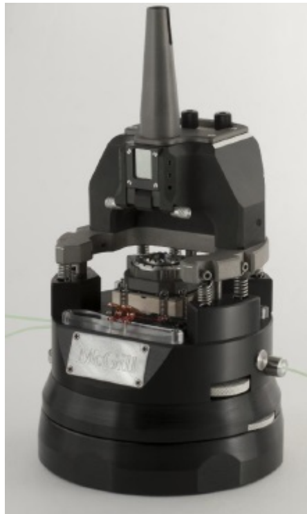
FIGURE A.1: The AFM used in this study without the photothermal attachment and a silicon cantilever holder.[24]
