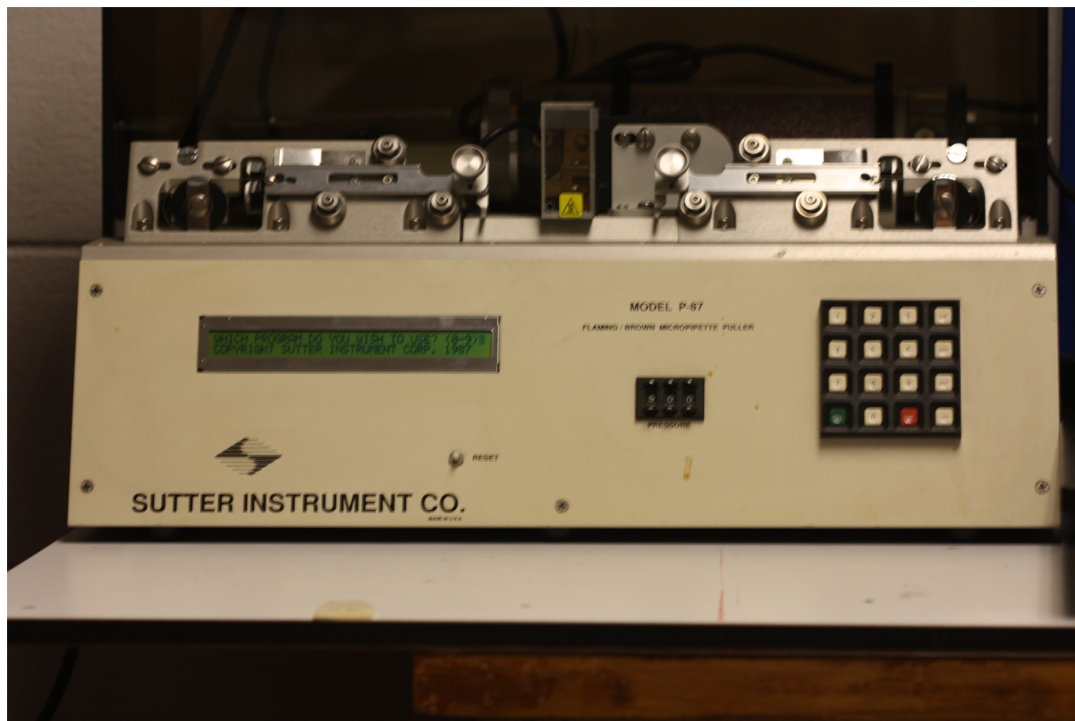
FIGURE 3.3: A P-87 pipette puller. The two metallic bars are brought towards the filament housing in the middle of the puller. The large round screws tighten the capillaries into place as they are pulled and heated simultaneously.
