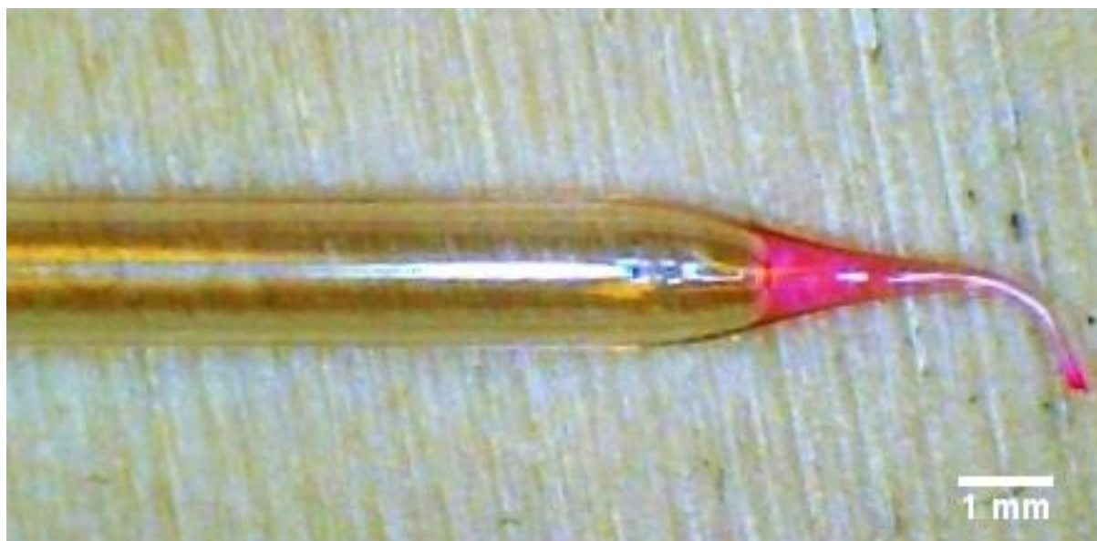
FIGURE 4.1: The first pipette probe was fabricated from a borosilicate capillary tube and was bent via the voltaic arc apparatus.
