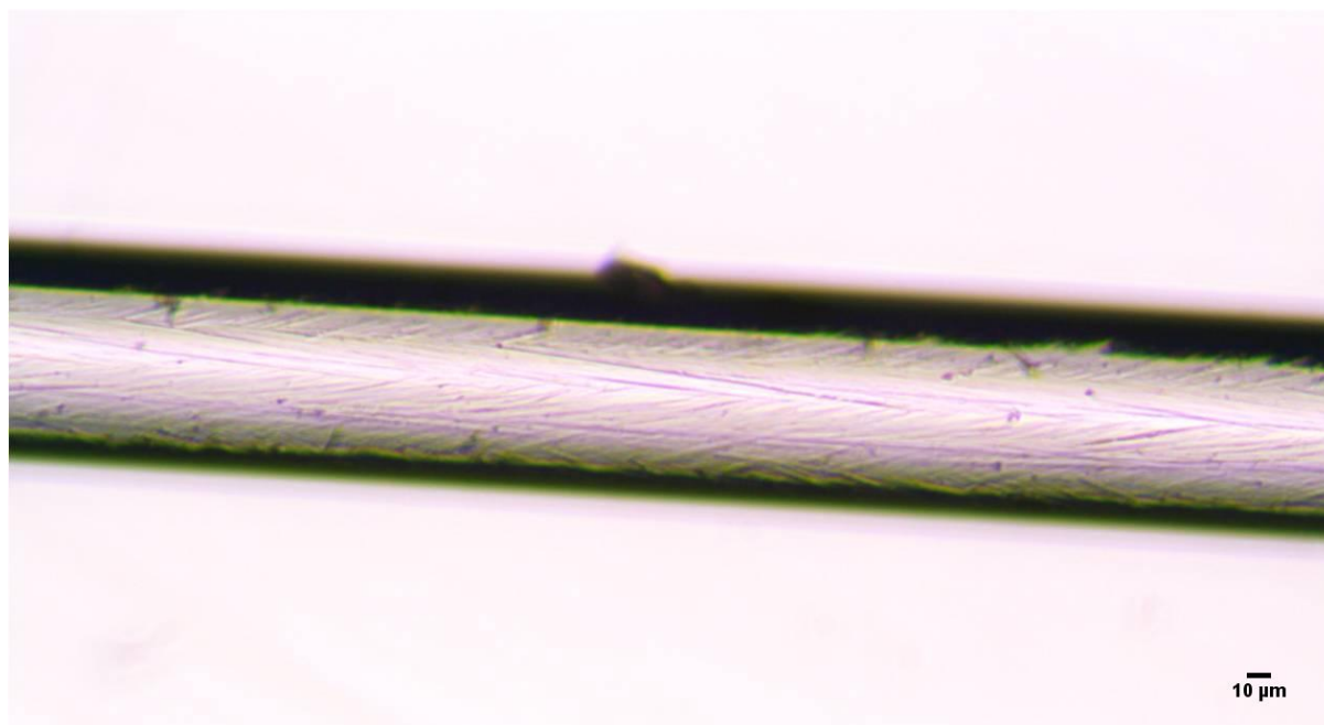
FIGURE 4.10: The scratches made through polishing this x-ray diffraction tube can be seen here. After the 5 micrometer grit polishing paper was used, progressively finer grits of polishing paper were used to smooth out the surface, although obtaining a smooth surface was not trivial.
