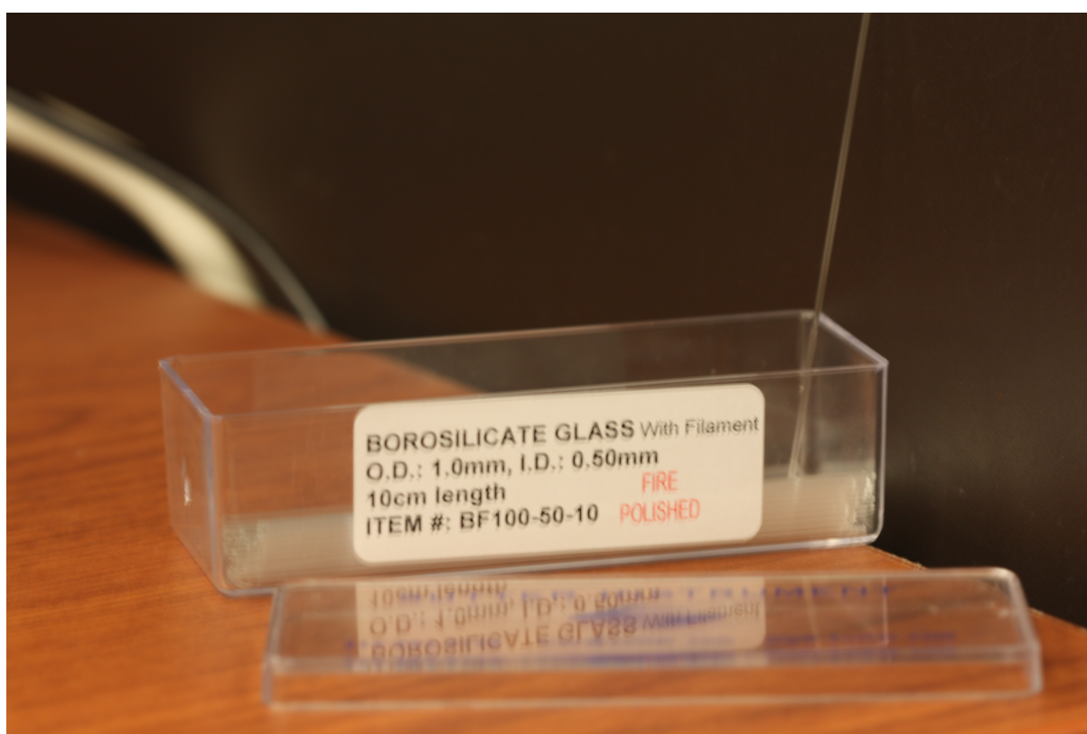
FIGURE 3.2: A borosilicate capillary tube is shown here with packaging. These capillaries are of outer diameter of 1.0 mm, inner diameter of 0.50 mm and a length of 10cm.
