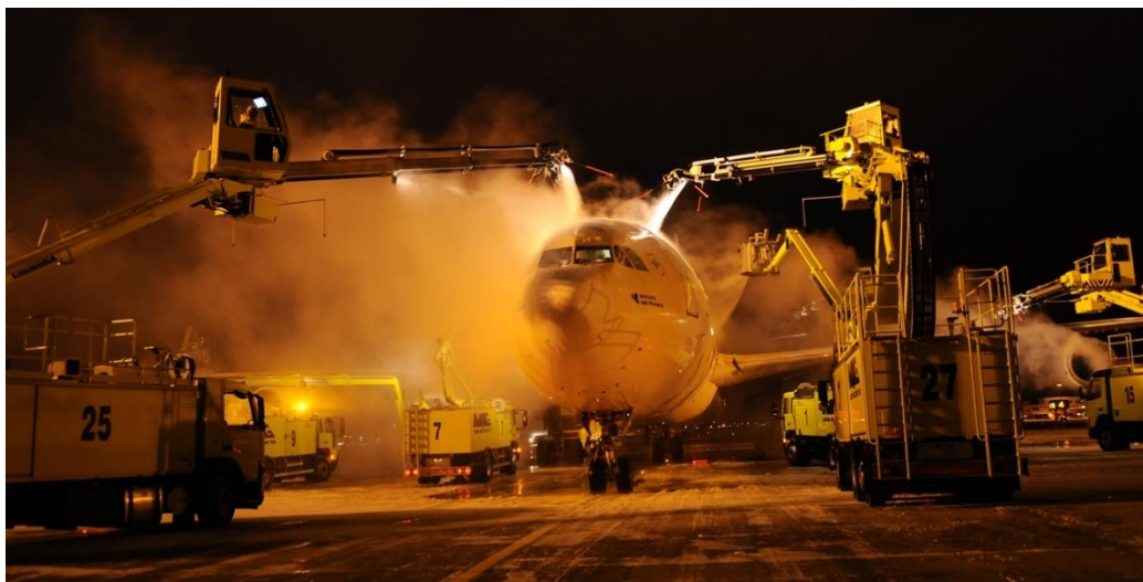
Figure 11—Modern De-Icing Equipment
