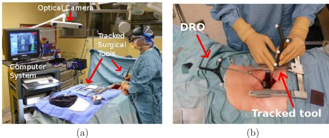
Figure 2-7: (a) The components of an image-guided surgery system consists of an optical camera, a computer system running a surgical navigation software, and the surgical tools with tracked target mounted on them. (b) The tracked surgical tools have reflective spheres mounted on them in uniquely identifiable configuration, known as tracked targets. All figures are reproduced and modified with permission from Goulet [7].
