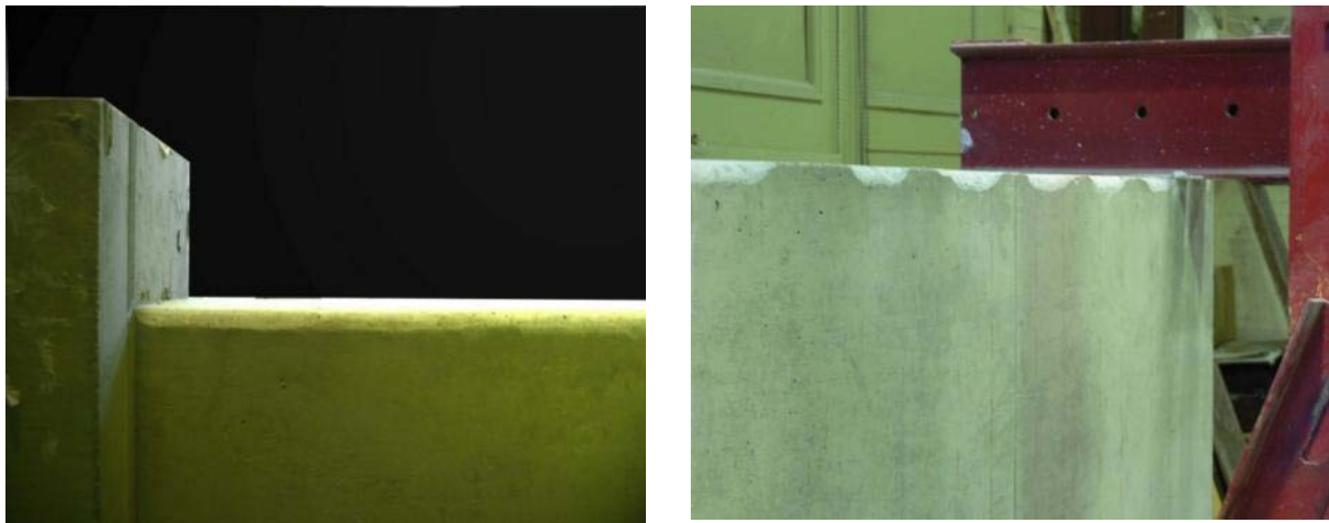
Fig. 2.5- Rounding the corners of the walls before installing the CFRP wrap
