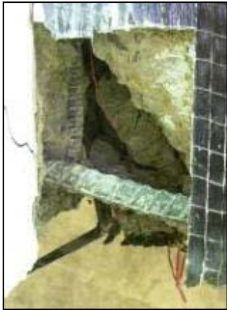
(b) Close-up view of concrete crushing and fiber rupture Fig. 3-23- Repaired walls at the end of testing
