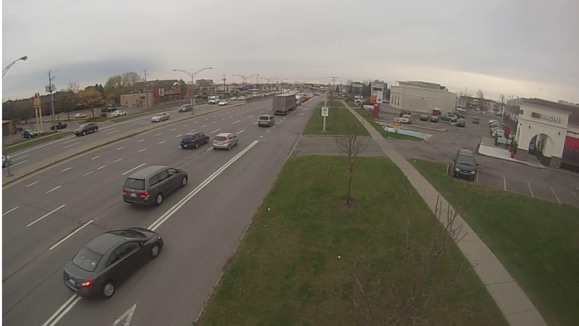
Figure 36 Typical behaviour during queuing, with a vehicle cross the pavement marking early
