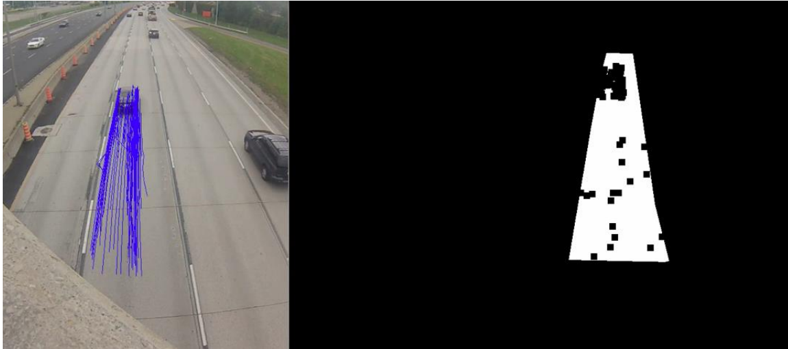
Figure 5 Trajectories being tracked along a lane (left) with the visible features appearing on the mask (right)
