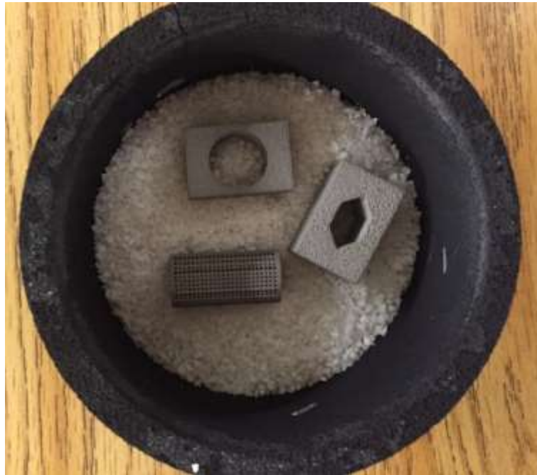
Figure 28: Sintering crucible with different parts
