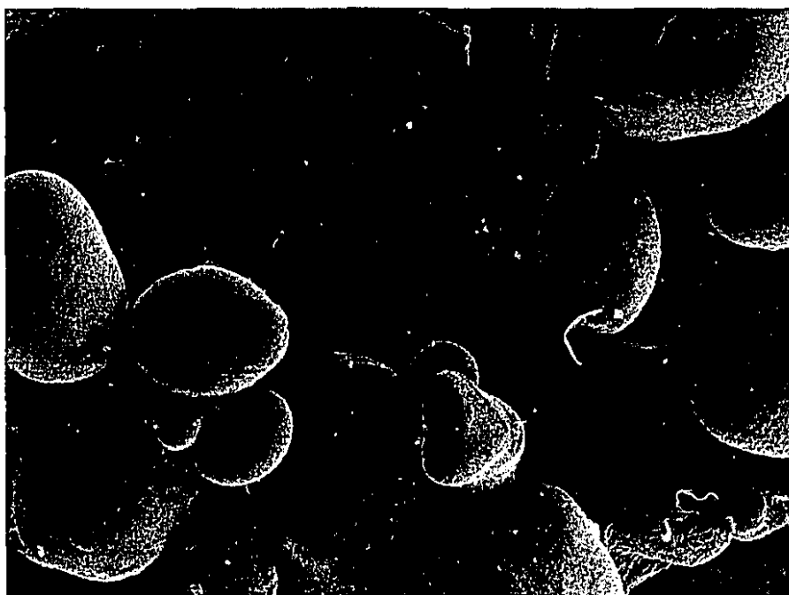
Figure 7.14 Scanning electron micrograph of potato tuber starch granules treated with UV radiation at 1.5 \times 10^4 \text{ W.s/m}^2 and hot water at 55^\circ\text{C} for 30 min.
