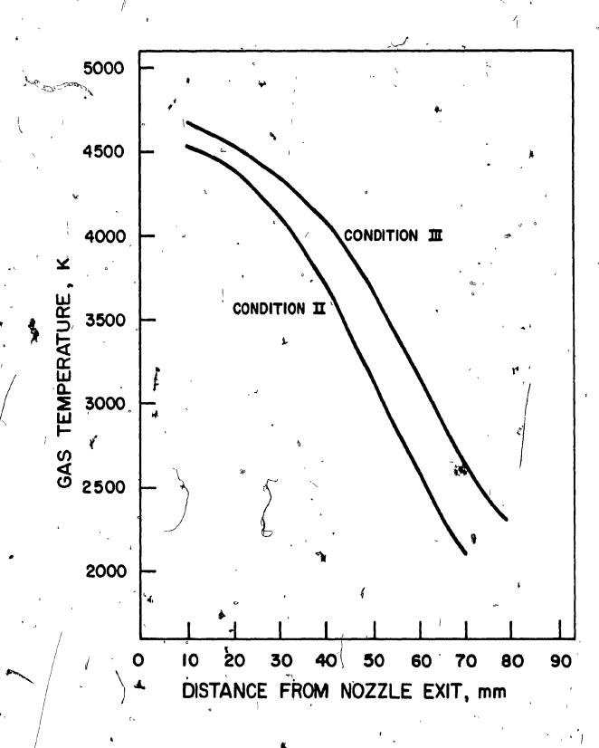
results obtained using Equations (25) and (26) were exactly the same for the gas velocity and within a fraction of a percent for the gas temperature. Tables III and IV list the temperatures and velocities calculated by the two equations, for two plasma operating conditions. This agreement reconfirms the concepts of using variable-property limiting Nusselt number and the reference temperature To.19 for evaluating the Reynolds number.
