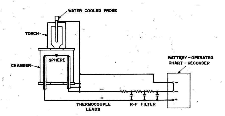
completely by the above-described method. However, it seemed that the potential attained by the probe was not exactly that of the gas. This difference in potentials manifested itself by sustained arcing in the upper sections of the chamber. An attempt was made to bring the thermocouple assembly to the gas potential by connecting it to the nozzle or the ground lead of the induction coil. These attemps, however, were even less successful in reducing arcing.
