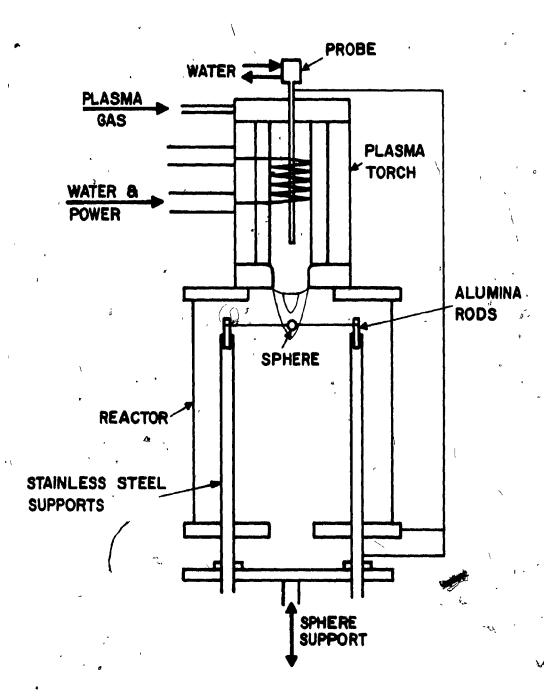
the flow of water in the annulus between the quartz tube and the outer Teflon jacket. The circulating water helped also in cooling the quartz tube, the gas distributor and the nozzle. The plasma gas, heated up and ionized in the coil section, left the torch as a low velocity jet through a constricting nozzle, 25 mm in diameter.
