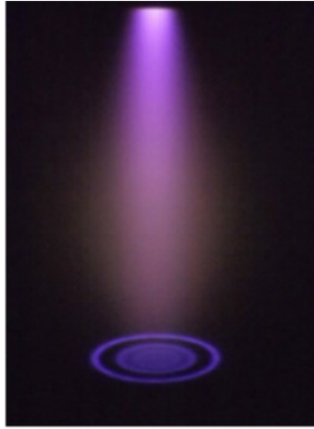
Figure 2: DC driven air glow discharge in a pin-water geometry with self-organization at the surface of the water anode electrode. 10
