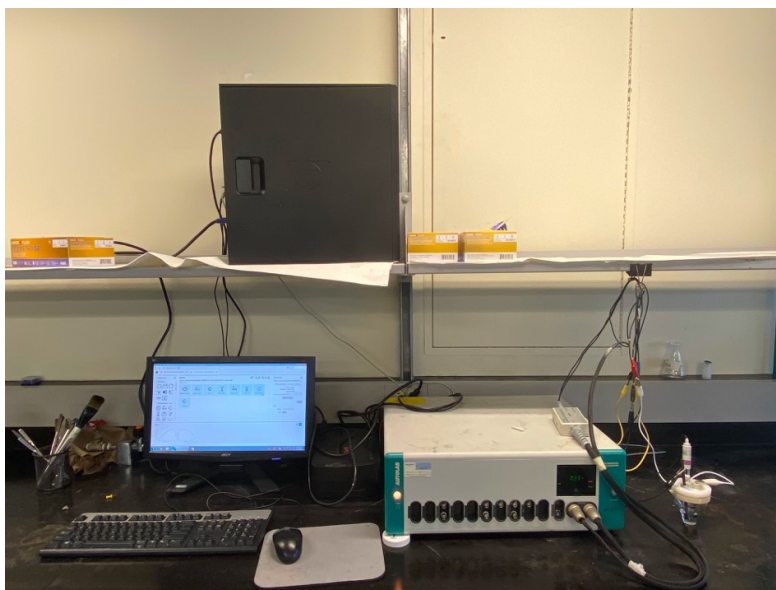
Figure 16: Full ASV setup. The electrical box on the right of the computer screen is the potentiostat (an instrument that applies voltage sweeps across electrodes). The glass funnel shaped beaker holds the PAW sample with the electrodes dipped into it. It is where the electrochemical reactions take place. The computer processes the electrical data and converts it into voltage and current plots based on what is desired. The electrochemical software used is NOVA from Metrohm Autolab.
