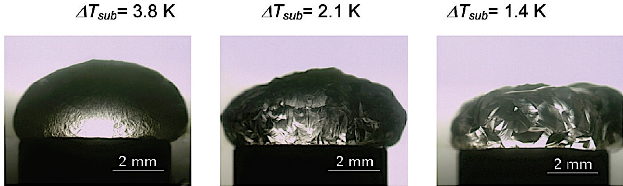
Figure 1.8. Morphology of gas hydrate at the liquid-gas interface in different subcooling conditions [20].
