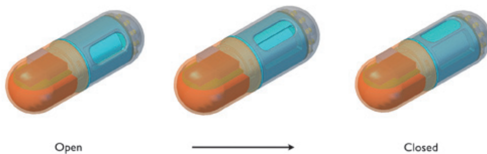
Figure 1: Illustration of basic rotary collection mechanism for GI sampling device
