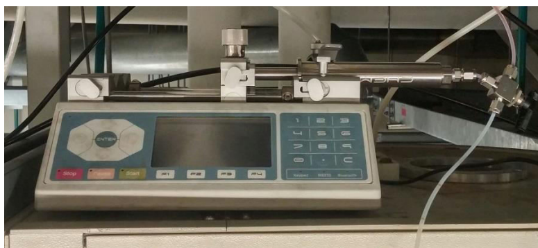
Figure 3-5: The liquid injection system based on a stainless steel syringe and a push-syringe.
