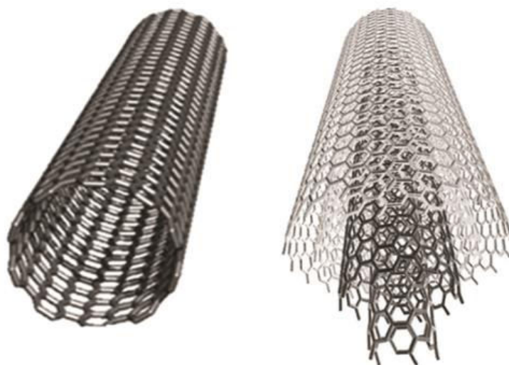
Figure 2-4: Representation of a single-wall (left) and multi-wall (right) carbon nanotube.
