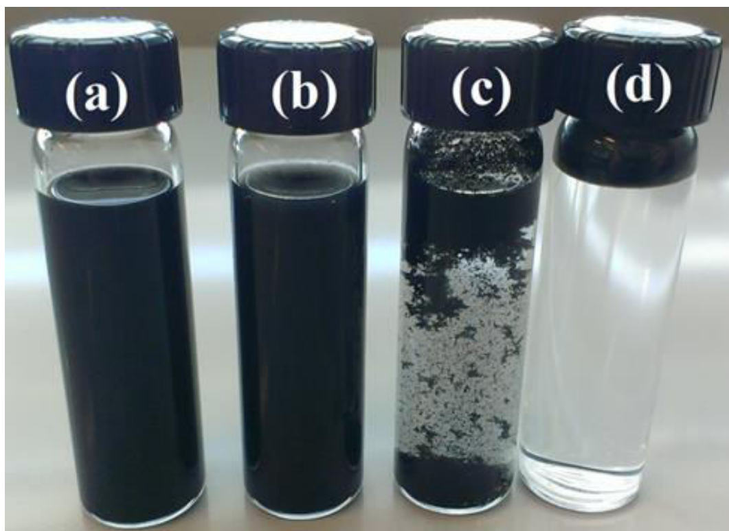
Figure 6-11. Observed stability after 6 weeks for a) O-GNFs with 14.2 at% Oxygen in ethanol b) O-GNFs with 14.2 at% Oxygen in water c) O-GNFs with 6.4 at% Oxygen in water and d) non-functionalized GNFs in water.
