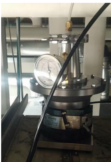
Figure 3-6: The powder feeder.
