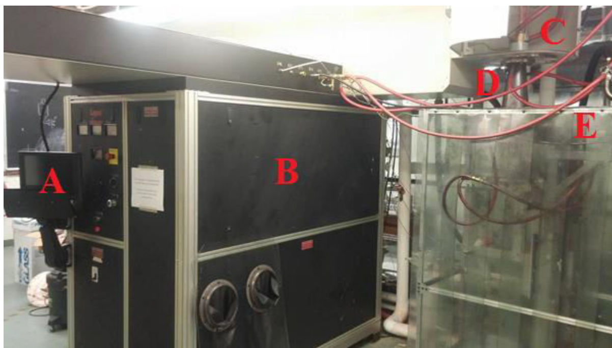
Figure 3-1: Picture of the experimental set-up. (A) control console (B) RF generator (C) ICP torch in the Faraday cage (D) conical reactor (E) exhaust connected to the vacuum pump.
