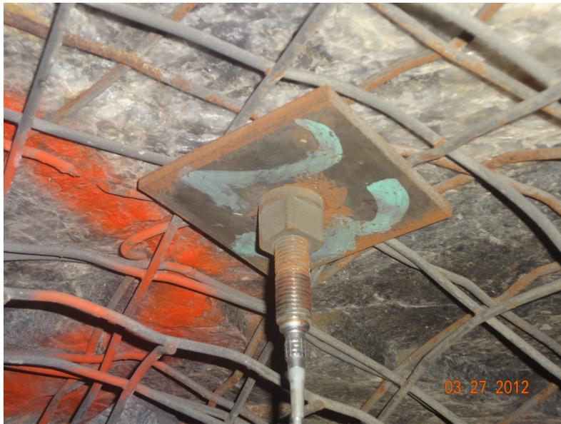
Figure A2-2 U-Cells in the drift wall and roof taking load
