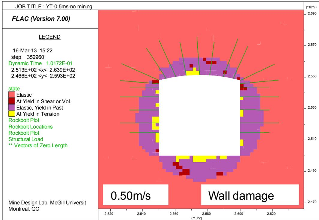
a) Wall damage around the drift for 0.5m/s PPV at the drift boundary
