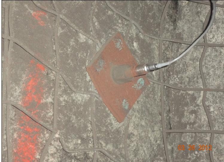
Figure5-5 Typical field installation of U-cell in a fully grouted rebar
