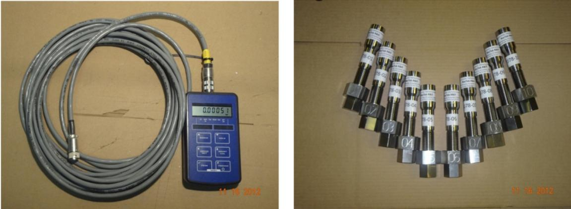
Figure 5-3 The U-cell portable readout unit and the new generation U-cells
