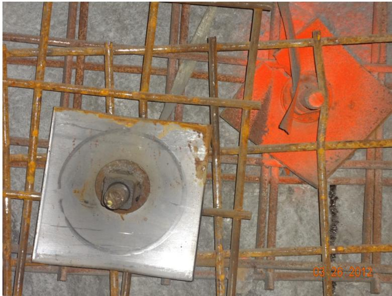
Figure A2-1 Cone bolt failing under shear force
