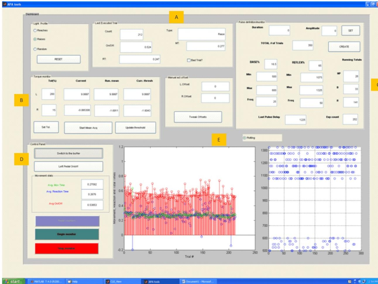
Figure 3.16. Graphical user interface (GUI) to monitor and control experimental parameters in real-time by interacting with SIMULINK block diagrams.
