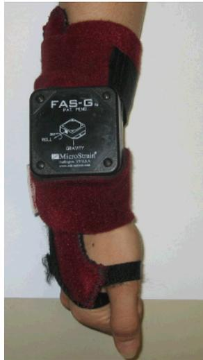
**Figure 3.8.** Inclinometer fixed with a wrist splint, used to measure angular arm position
