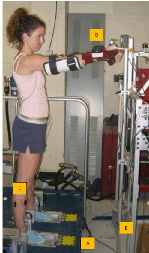
**Figure 3.1.** A typical subject executing a voluntary arm movement while standing on the actuator. A) Bilateral electro-hydraulic actuator fitted with two foot pedals and torque, position and load transducers. B) Aluminum target frame holding visual and audio cues, torque feedback meter and target switch. C) Surface EMG electrodes on postural and focal muscles. D) Inclinometer used to measure arm position.
