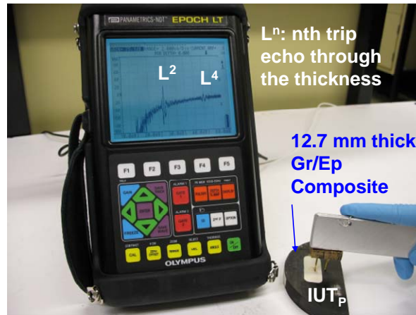
Figure 2-63 Measurement setup for the IUT_P shown in Figure 2-62 at room temperature using an EPOCH LT.
