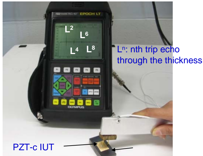
Figure 2-8 Measurement setup for an IUT made of PZT-c film using an EPOCH LT in pulse-echo mode.
