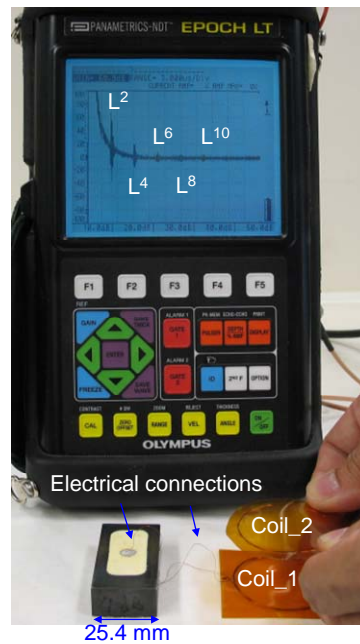
Figure 5-27 An IUT deposited onto a 12.7 mm thick steel plate measured by a non-contact configuration using an EPOCH LT. The two ends of Coil_1 are connected to the top and bottom electrodes of the IUT directly, and there is no ferrite on Coil_2, which is different from the one shown in Figure 5-26. In this experiment D_{avg} = 5 cm, n = 5 and d_{avg} = 4 cm.
