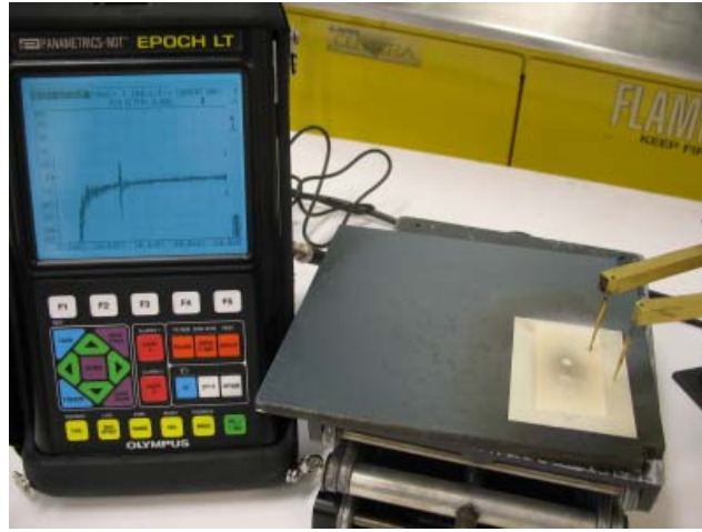
Figure 2-69 IUTs deposited onto a 6.9 mm thick Gr/Ep composite plate having impact damages.
