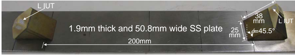
Figure 4-35 The experimental setup for the S_Y wave in the wedge to excite and receive PAWs in the SS plate.
