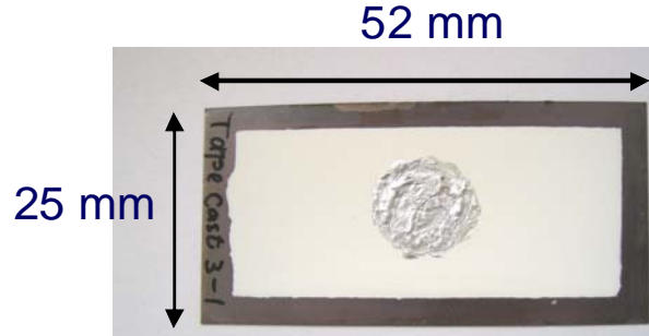
Figure 2-44 Photograph of a a 50 \mu\text{m} thick PZT film coated onto a 75 \mu\text{m} thick SS membrane by tape casting.
