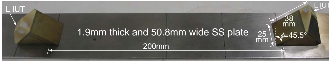
Figure 4-33 Experimental setup for the L wave in the wedge to excite and receive PAWs in the SS plate
