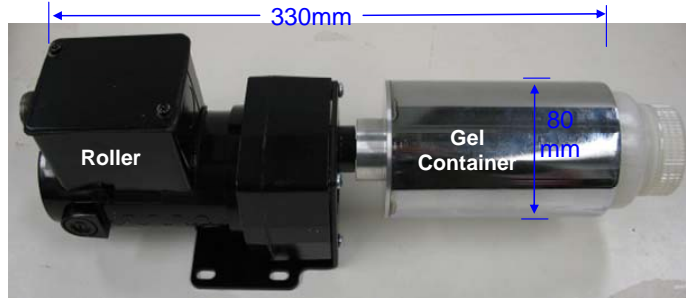
Figure 2-3 Ball milling of the mixture of powder and sol-gel solution in Figure 2-2. The second step of sol-gel based UT fabrication process shown in Figure 2-1.
