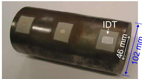
Figure 4-50 A steel tube with 102 mm external diameter and 46 mm inner diameter and IDT for SAW generation and detection in pulse-echo mode.
