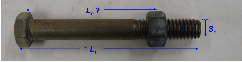
Figure 3-24 Schematic diagram for the axial load measurement.
