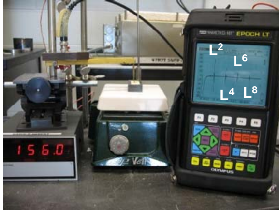
Figure 2-17 Measurement setup for an IUT made of PZT-c film at 156°C using an EPOCH LT.
