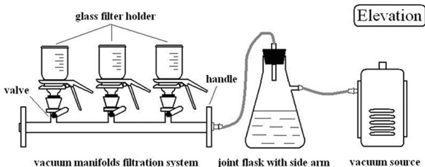
Figure S2.2: Multiple manifold vacuum pump set-up for regular filtration
