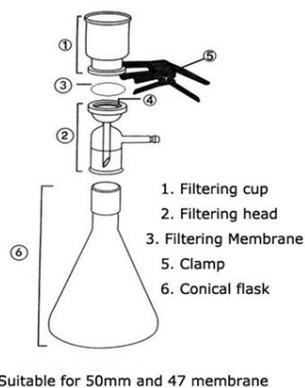
Figure S2.3: Vacuum filtration apparatus set-up after oil separation or for faster filtration.
