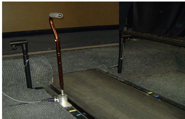
Figure 3-2: View of the instrumented cane with ball-joint base, affixed to left side of the self-paced treadmill.
