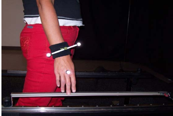
Figure 3-1: Haptic strip with embedded load sensor, placed at fingertip height.
