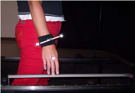
Figure 4-1: Instrumented devices used in the study. (A) Haptic strip embedded with load sensor placed at fingertip height. (B) Instrumented cane device with ball joint base affixed to left side of the self-paced treadmill.
