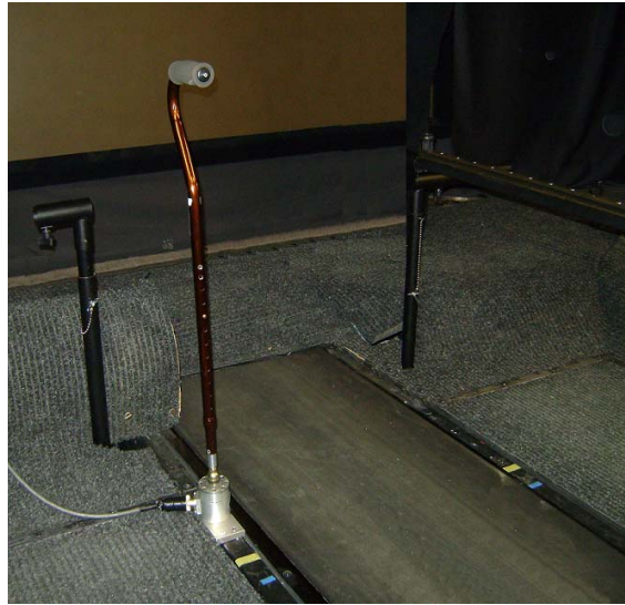
Figure 4-1: Instrumented devices used in the study. (A) Haptic strip embedded with load sensor placed at fingertip height. (B) Instrumented cane device with ball joint base affixed to left side of the self-paced treadmill.
