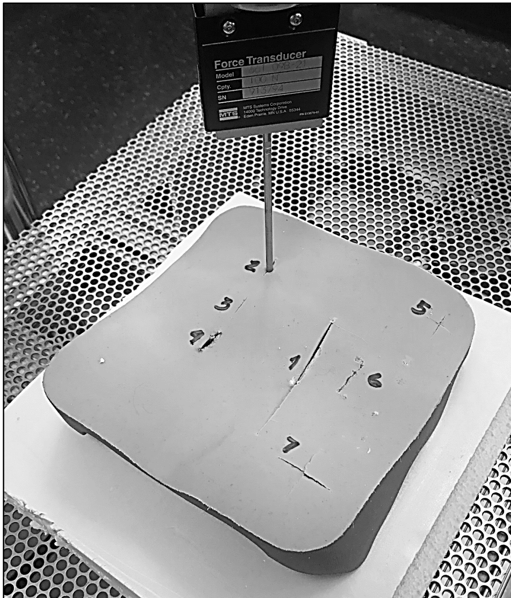
Figure 4-9: Experimental setup of physical interface showing the order of the incisions (1–7)
