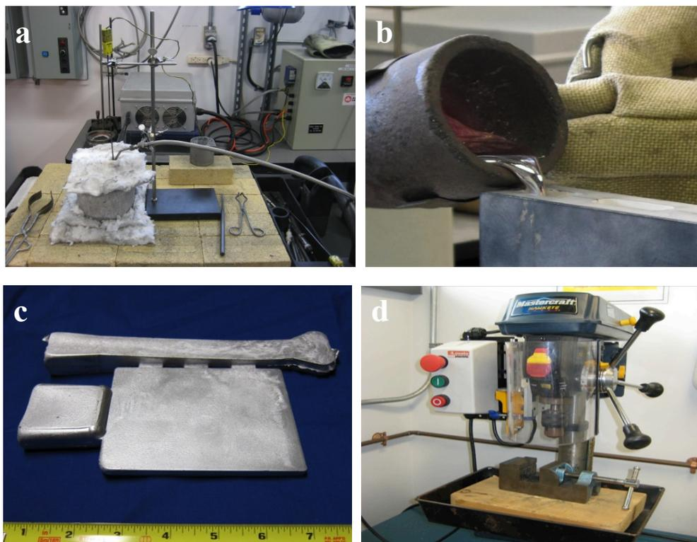
Fig. 3. 1. Casting procedure: (a) melting in graphite crucible with induction furnace, (b) pouring the melt into the preheated die, (c) thin plate cast sample, (d) drill used to obtain the chips.
