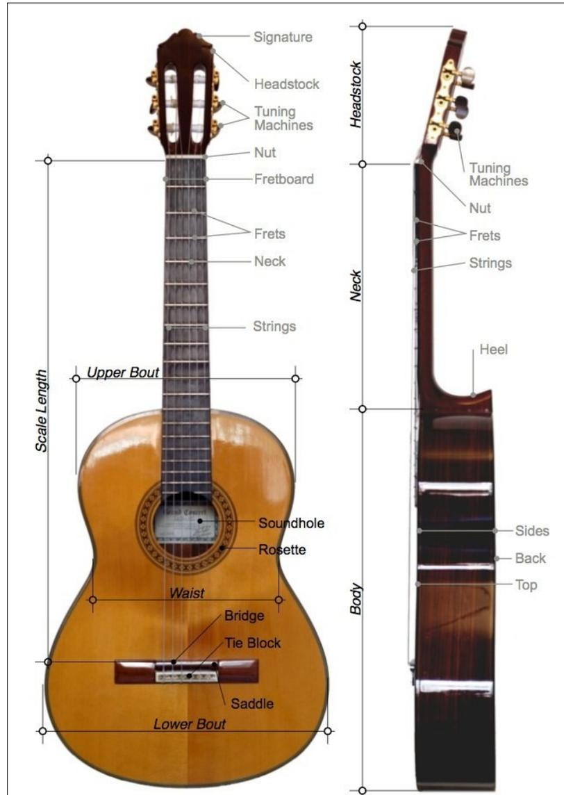
**Figure 1-3:** Parts of the guitar [11]
