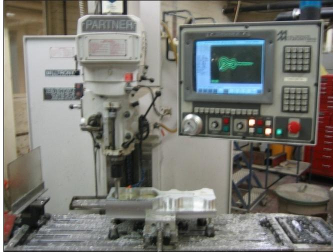
**Figure 5-6:** CNC machining of prototype mould
