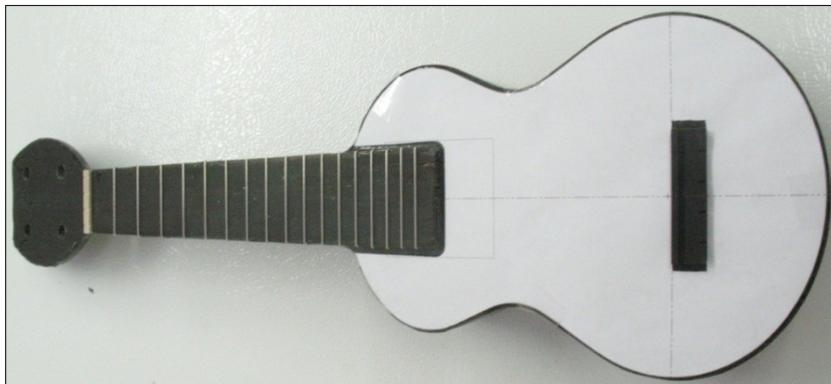
**Figure 7-4:** Template used for attaching the bridge
