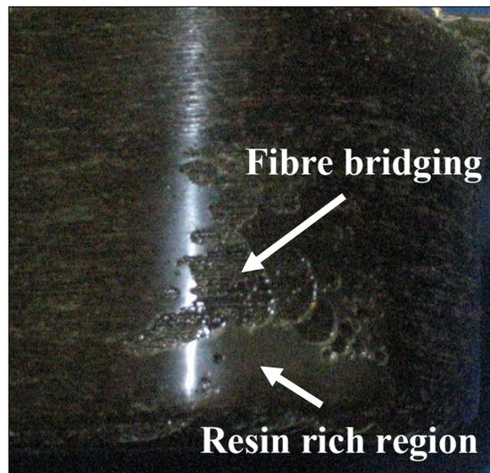
**Figure 6-12:** Recurring defects on prototypes
