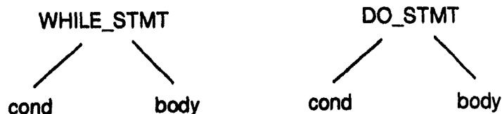
Figure 2.10: The SIMPLE AST for WHILE_STMT and DO_STMT.
