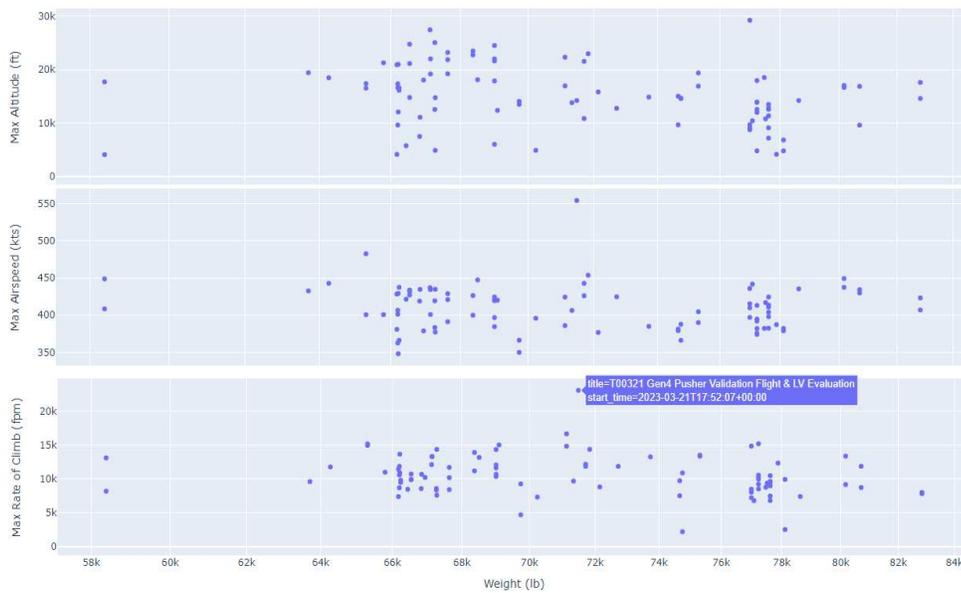
**Fig. 4.13:** Aircraft Weight vs. Max Altitude, Airspeed, and Rate of Climb
