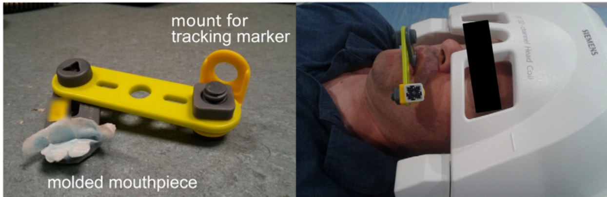
Figure 2.6: Optical tracking system for prospective motion correction from Todd et al. [2]. (Reproduced in accordance with the associated Creative Commons CC-BY Licence.)
