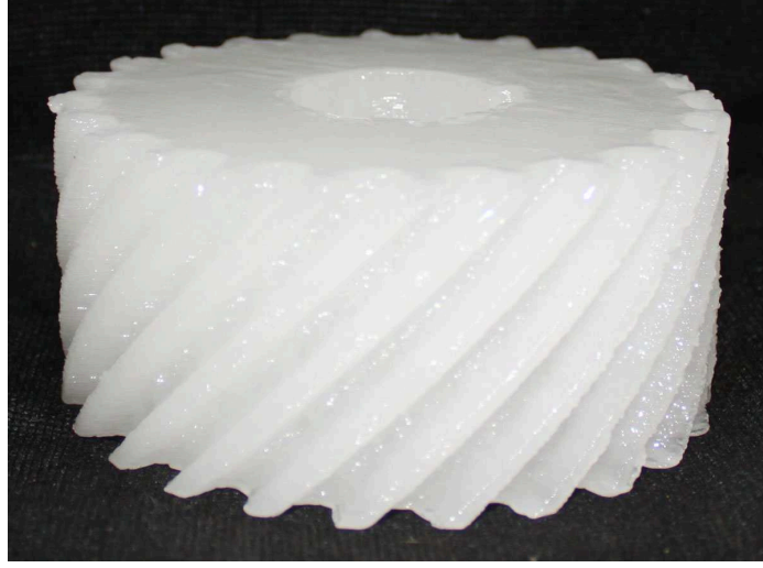
Figure 5–7: The final helical ice gear, constructed with SMF, after the scaffolding is removed
