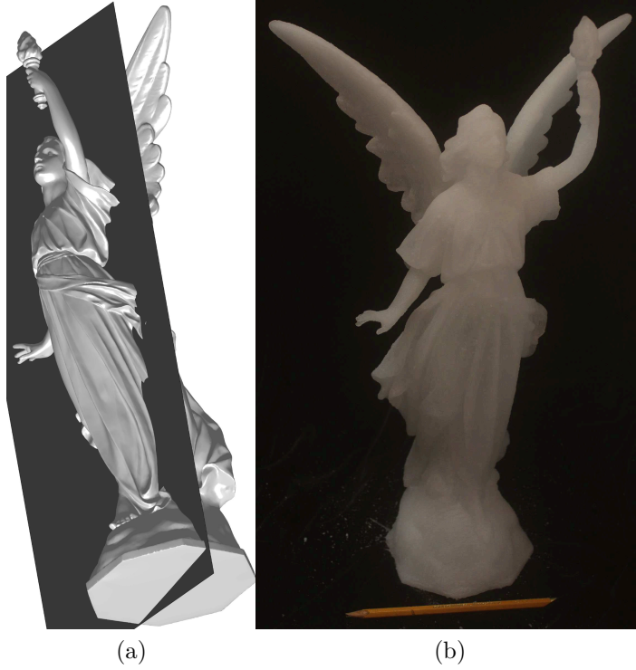
Figure 4-10: (a) STL file courtesy of the Stanford 3D Scanning Repository, produced by scanning a statue of Lucy, a Christian angel; (b) the ice statue, 0.5 m high, built with the Cobra 600 rapid freeze prototyping system
