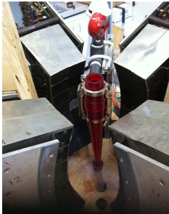
Figure 4.10: The two-inch hydrocyclone inside the modular camera assembly (overflow piping removed for picture clarity).
