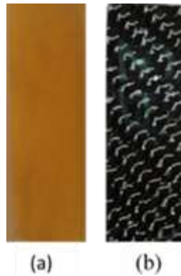
Figure 7.1 Samples for water absorption test (a) epoxy-based resin (matrix) (b) FRP shell
