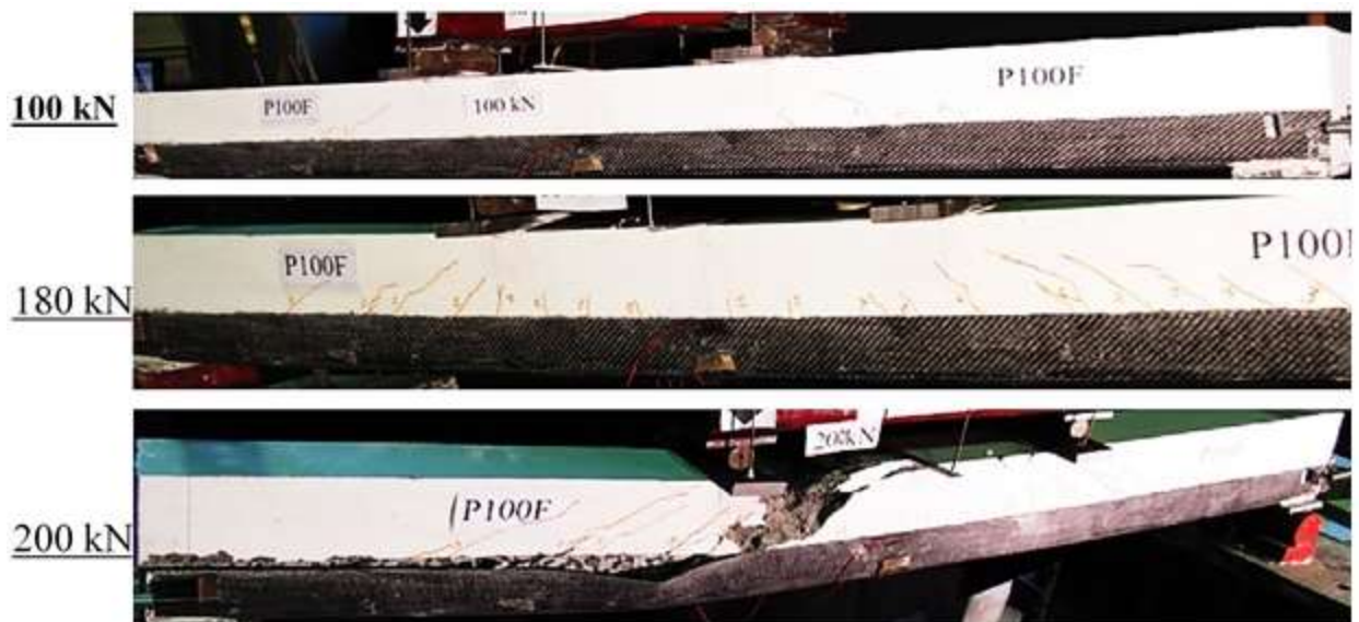
Figure B.1.2 Failure modes of Beam P100F
