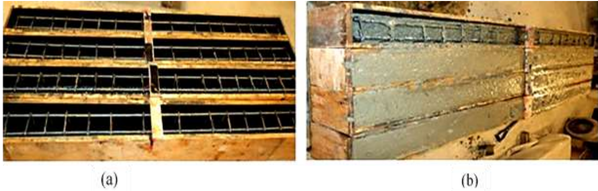
Figure 5.3 Specimens construction (top views) (a) ready for concrete casting (b) during pouring of concrete
