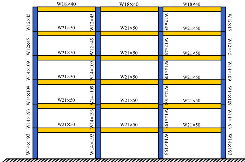
Figure 3-5 Schematic of building structural sections
