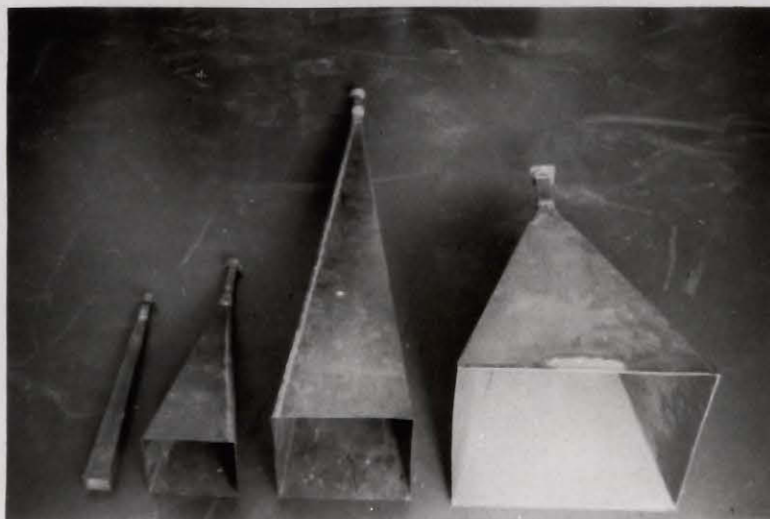
(c): From the left: the small horn used in lens illumination, and the 10, 15, and 26 \lambda horns.
