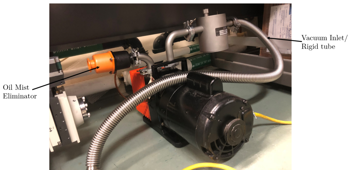
Figure B.1: An image of the vacuum pump showing the oil mist eliminator at the pump outlet and the rigid tubing leading to the pump inlet.
