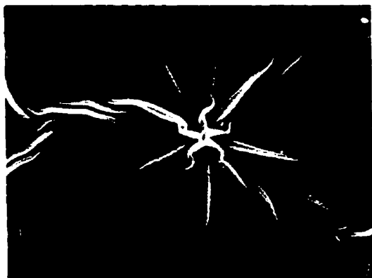
Figure 7. 3 Laser-induced changes in silica-methacrylate thin film
