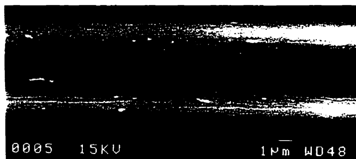
Figure 6. 1 Scanning electron micrograph of self-inscribed channel waveguide, showing striations parallel to the waveguide long-axis.
