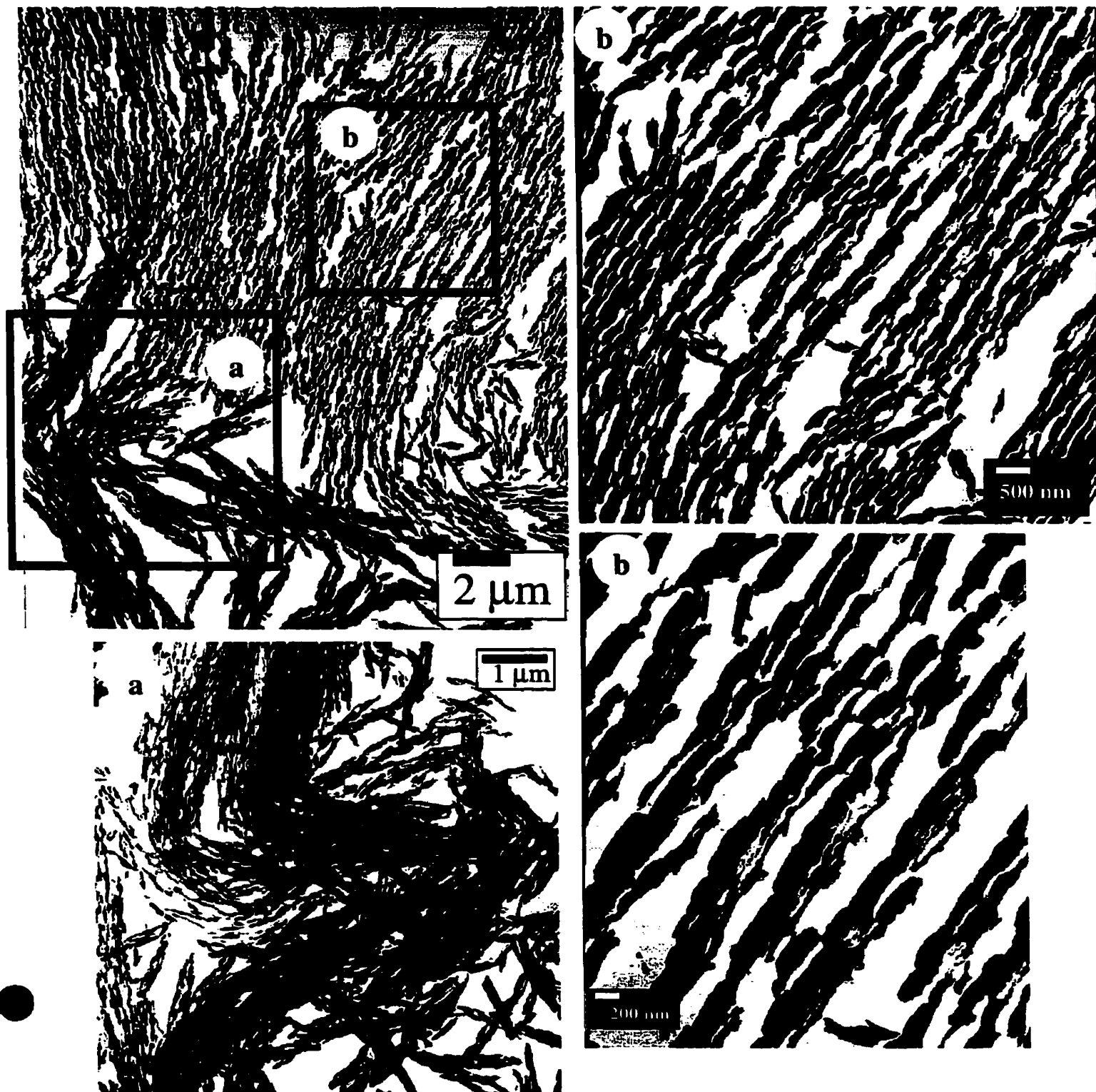
Figure 5. 19 Cross-sectional transmission electron micrographs of SAC-01 composites that had been heated at 700 °C for 10 hours
